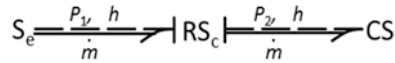
Fig. 8.4 A tank being charged with a fluid from a source through a restriction
