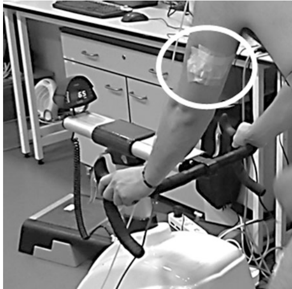
Fig. 3.1 Thermal contact sensor attached to the skin during cycling (inside the circle)
