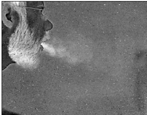
Fig. 2.6 Infrared camera with detector for visualizing the middle infrared, and then the CO 2 exhaled in the respiration. Figure extracted from Walther and Weimann [17]
