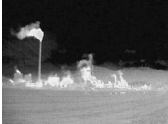
Fig. 1.9 Thermography of the gas emission in a paper factory. Figure obtained from Sedláč et al. [28]
