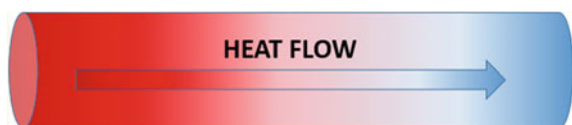
Fig. 2.1 Heat flow: the heat is transferred from the hotter side to the cooler
