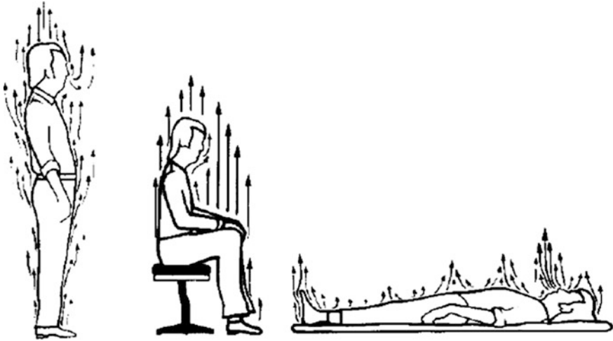
Fig. 3.12 Effect of the body posture on the heat flow. Figure obtained from Houdas and Ring [66]
