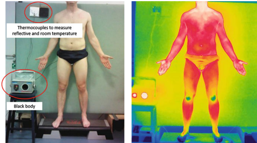
Fig. 3.6 Examples of different references (black body and thermocouples) placed in the space of measurement to increase the reliability
