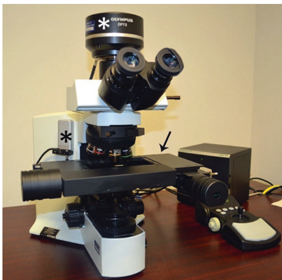
Fig. 11.12 Live microscope setup for stereology. The microscope contains a camera (white asterisk), motorized stage (arrow) and length gauge (black asterisk)
