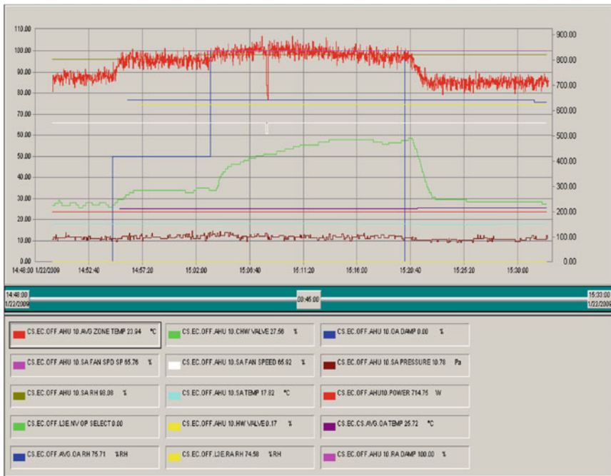
Fig. 4 An example of the sensor data for an air handling unit in the Newcastle building
