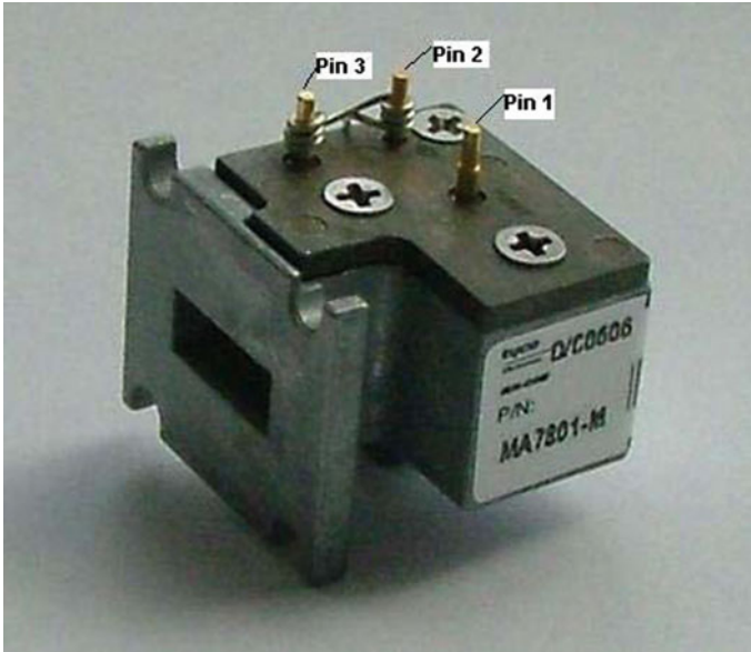
Fig. 12 MACOM MA 7801-M Mono-Doppler transceiver used in this experiment. Operating frequency is 24.1 GHz
