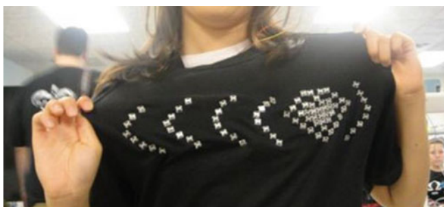
Fig. 1 T-shirt with pulsing LED related with wearer heart beat
