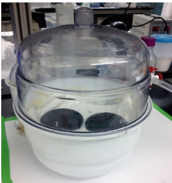
Fig. 8 Desiccation of the PDMS nanocomposite
