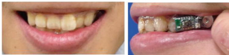
Fig. 15 Photographs ( front- and side-views ) of invisible “Smart mouth gear” for monitoring salivary glucose. The mouthguard biosensor to custom-fit the patient’s dentition. The device consisted of a glucose sensor and wireless BLE transmitter incorporating a potentiostat for stable glucose measurement. The wireless transmitter was neatly encased in PETG mouth guard material
