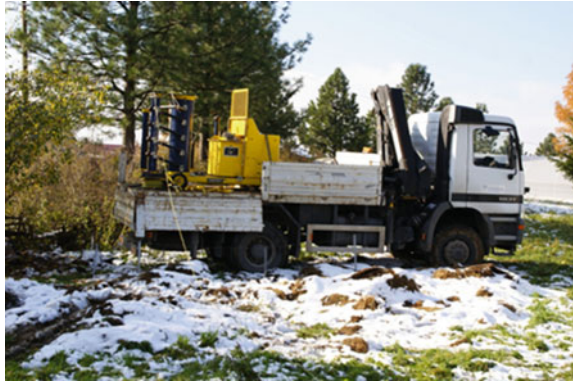
Fig. 6 Position of impulse generator during testing
