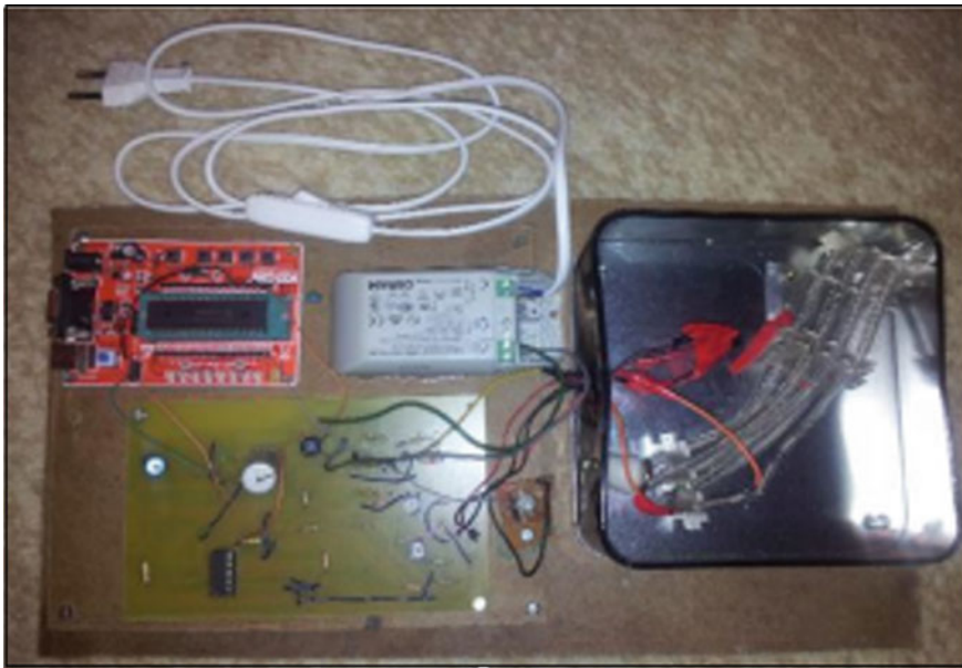
Fig. 5 Appearance of the finished system for closed-loop temperature control
