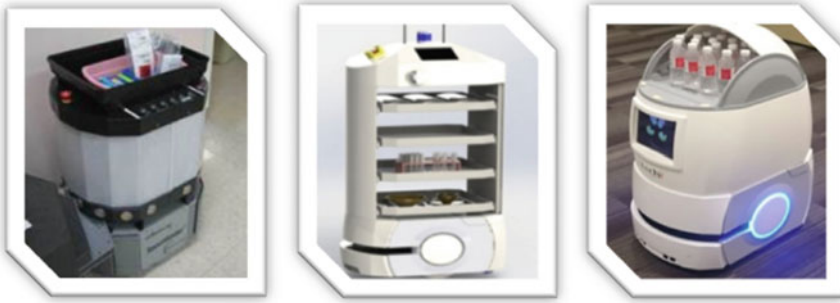
Fig. 15 The robotic courier system used in medical institutions to serve patients [1]
