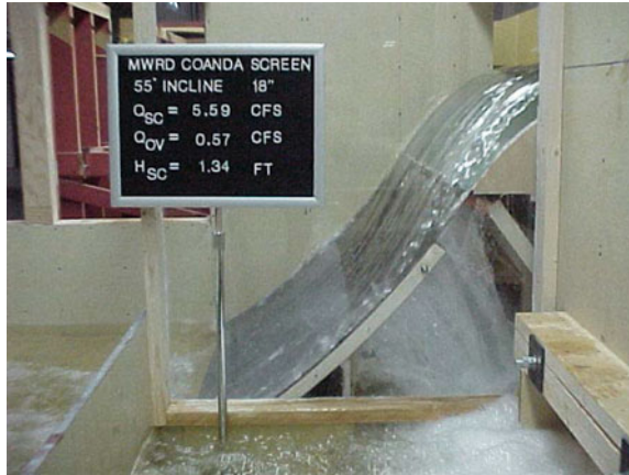
Fig. 2 The Coanda-effect screen tested in the hydraulic laboratory. Source [2]
