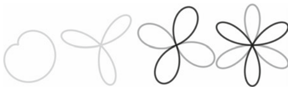
Fig. 10 Combined ( left ) and plain ( right ) multipoles of low orders
