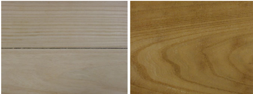
Fig. 4 Left paulownia, quarter-sawn (top) and flat-sawn (bottom). Right: flat-sawn catalpa, part of an unfinished qin back plate (Author photographs)
