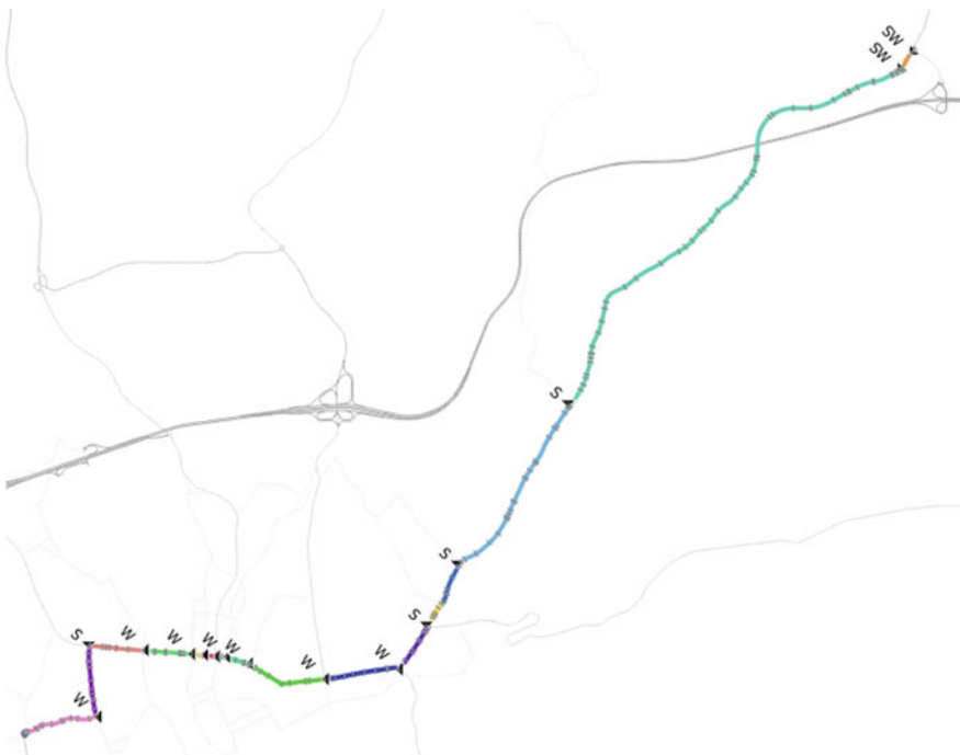
Fig. 7 Sections of the road 'B1—Wiener Straße' between junction to 'Kreisel Eugendorf A1' and junction to 'B1—KV Hans Schmid Platz'. The different colors represent the different Sections . The short grey lines reveal the Segments . The black arrows and letters indicate the driving direction of the sections as Cardinal Direction
