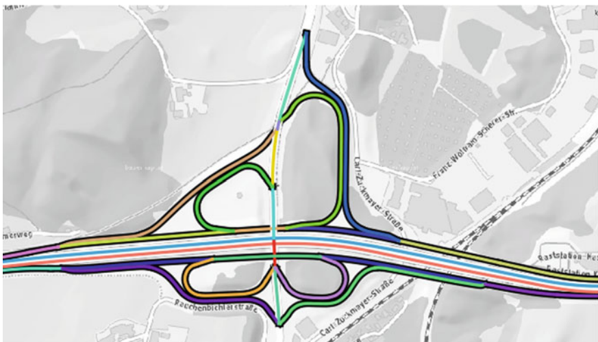
Fig. 6 Sections of junction “A1—Westautobahn—Anschlussstelle Salzburg Nord”. Each section is illustrated in a unique colour, and Ramps are marked with a black solid outline
