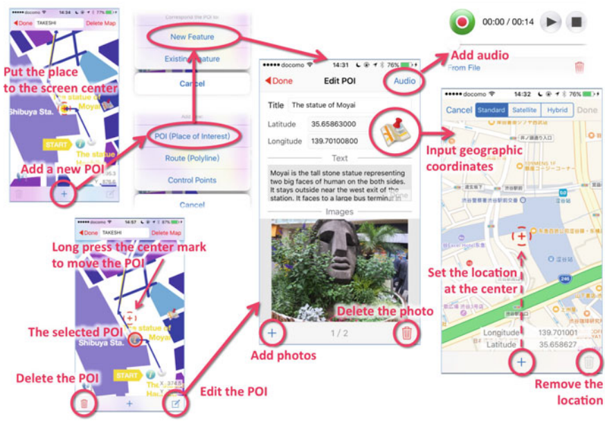
Fig. 4 Steps and interfaces of inputting a POI on a hand-drawn map using Manpo (the iPhone version used by the students in 2015)
