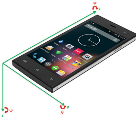
Fig. 1 Smartphone coordinate system and corresponding orientation angles. Pitch (theta) is the rotation around the width axis ( y ) relative to the horizontal plane, roll (phi) is the rotation around the height axis ( x ) relative to the horizontal plane, and yaw is the rotation around its depth axis ( z ) relative to geographic north
