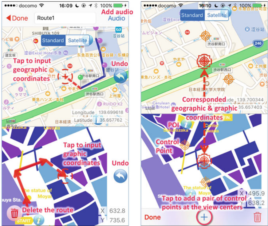
Fig. 5 Interfaces of inputting routes (left) and additional control points (right) on a hand-drawn map using Manpo (the iPhone version used by the students in 2015)
