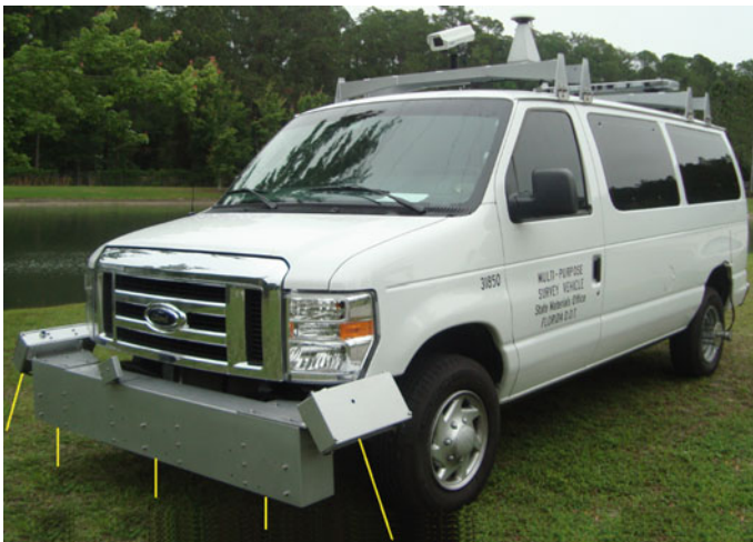
Fig. 5 MPSV with a 5-point laser sensor setup
