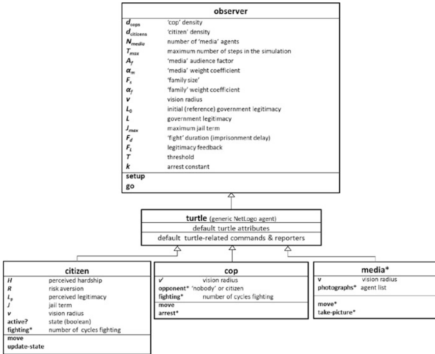
Fig. 1 Class diagram for all agent types in the NetLogo implementation. In NetLogo, agent types are implemented as subclasses of a generic ‘turtle’ class via the breed primitive. Agent types, attributes, and methods that are extensions of Epstein’s model are marked by an asterisk
