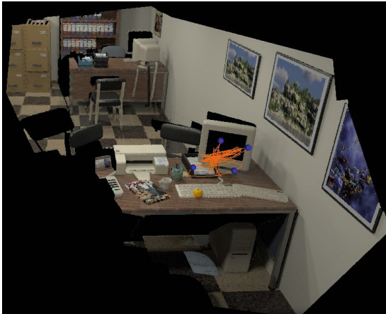
Fig. 7. Dense map built using depth maps of keyframes. The trajectory is drawn in orange and keyframes are blue spheres. (Color figure online)
