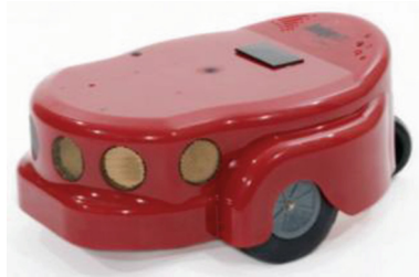
Fig. 1. Amigobot: differential-drive robot by Adept MobileRobots used in this work.
