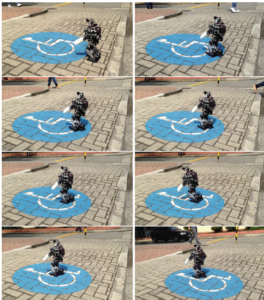
Fig. 9. Robot climbing an accessibility ramp.
