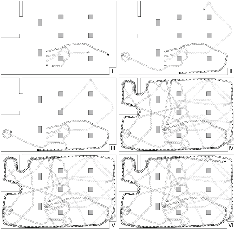
Fig. 8. Experiment 3: Introduction of a new team member and occurrence of a robot total failure. With a new member, robots are enumerated r_0 (black trails), r_1 (gray trails), r_2 (light gray trails), and r_3 (gray trails), from top first position to bottom. In frame I, r_0 , r_1 , and r_2 execute the available tasks. Frame II shows r_2 failure. The new team member, r_3 activates the behaviors set in frame III. In frame IV, both wander-side tasks are complete. So, r_0 finishes its task in frame V. Also r_0 activates REPORT and finishes the mission, as showed in frame VI.
