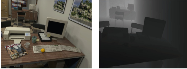
(a) RGB image loaded from the dataset. This is a synthetic environment with small camera motions around the desk. (b) Depth map loaded from the dataset. It is used just for keyframes
