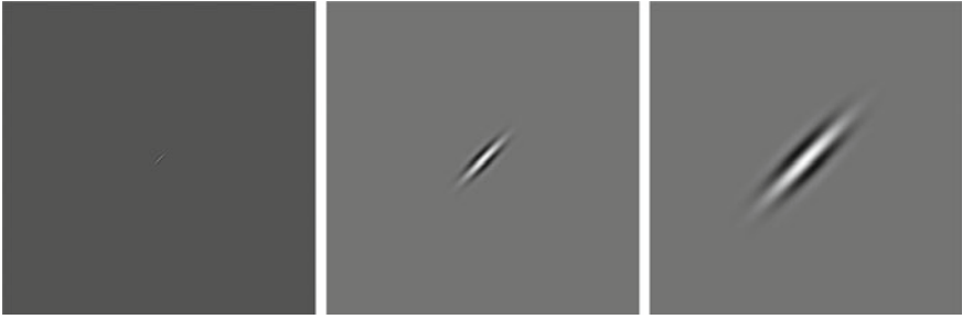
Fig. 1 Gabor filter kernels of size 300 \times 300 pixels with l = 2.5 , \theta = 45^\circ and using \tau = 5 , \tau = 10 , and \tau = 20 pixels, respectively
