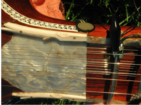
Fig. 7 FSR sensor used to measure thumb pressure
