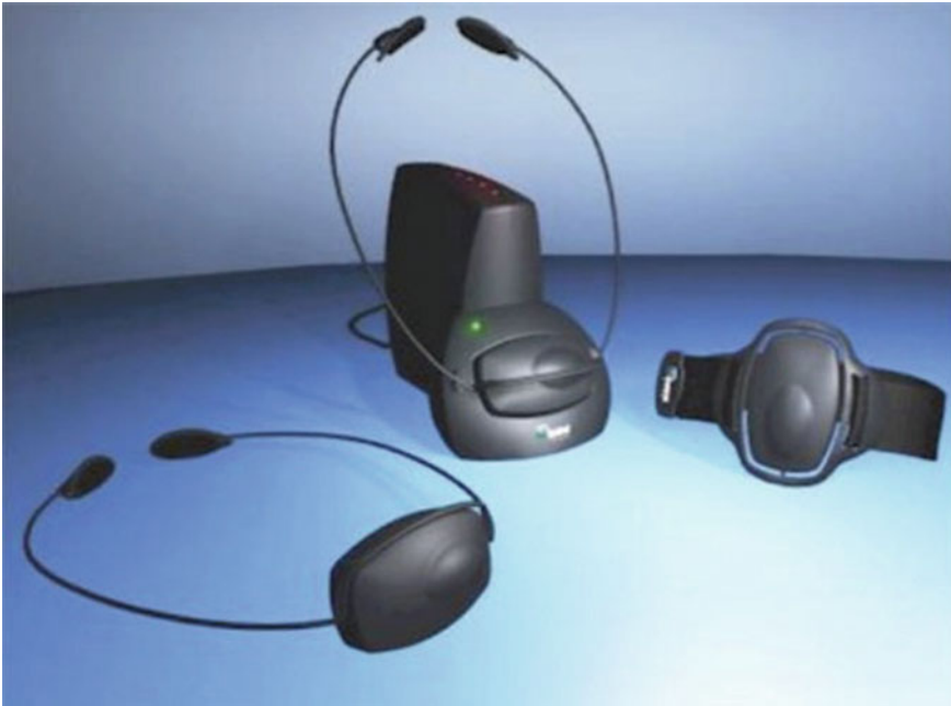
Fig. 1 EMG and gyro-based position controller: arm bands, head bands, and base
