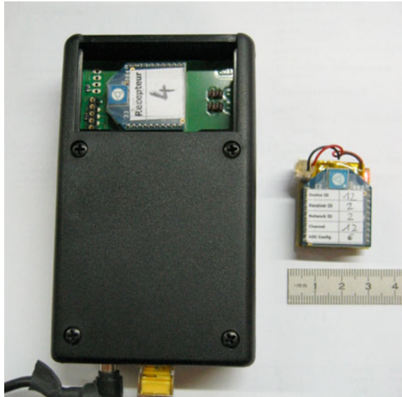
Fig. 1 Right the module with Xbee, battery and sensors (on the back of the module). Left receptor, showing the Ethernet and power supply connectors
