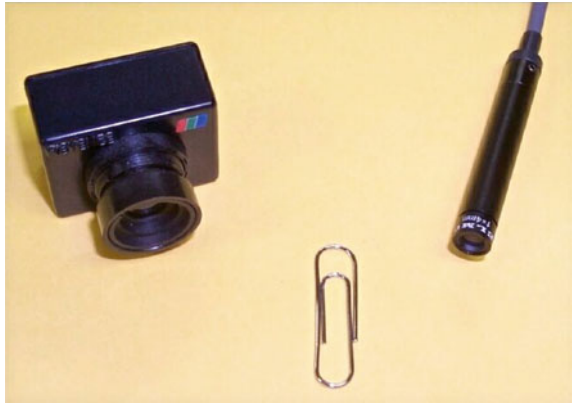
Fig. 3 Two miniature CCD cameras used in this work
