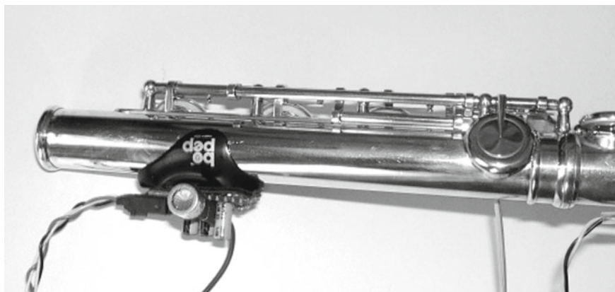
Fig. 3 Accelerometer and ultrasound transducer mounted on a Bo-Pep
