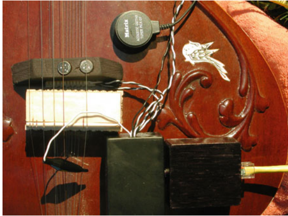
Fig. 6 Gesture capturing sensors at base of the ESitar
