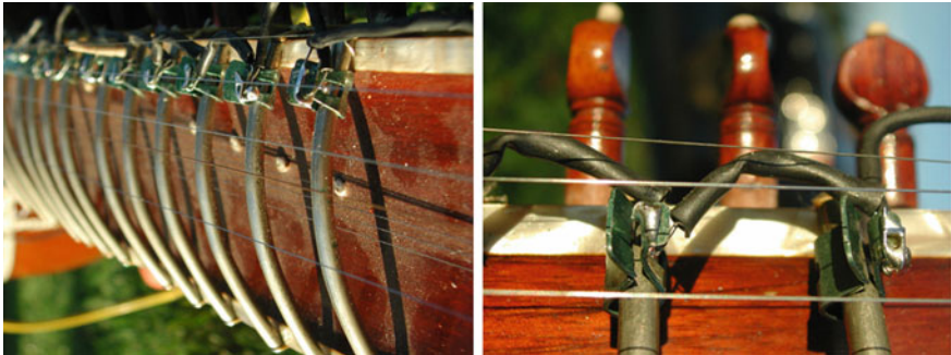
Fig. 5 Network of resistors on the frets of the ESitar
