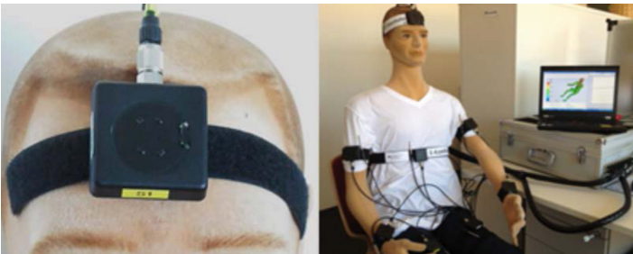
Fig. 1. Equivalent temperature sensor and system software of DressMAN 2.0
