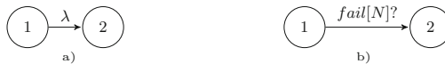
Fig. 9. Principle of converting a Markov model (a) to an STA model (b). N identifies a generator producing a fault the edge is sensitive to
