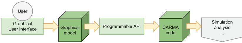
Fig. 1. A flowchart depicting CARMA code generation from graphical input.
