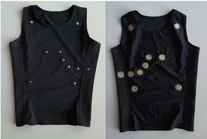
Fig. 2. The Shenzhen Yingda Strong Technology ECG T-Shirt - right and left side.
