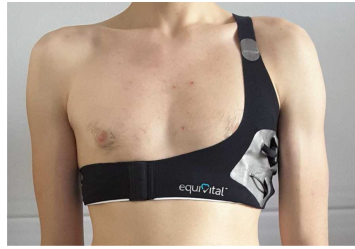
Fig. 4. EQ02 LifeMonitor elastic band with 3 textile electrodes.
