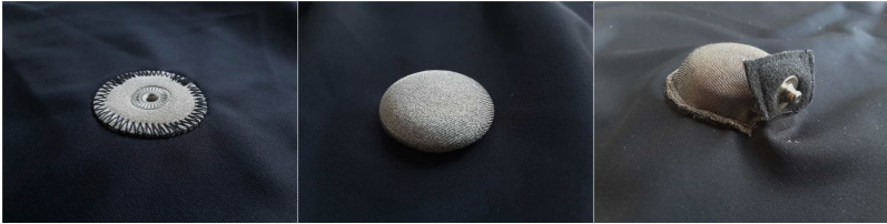
Fig. 5. The textile electrodes from: Shenzhen Yingda strong technology ECG T-Shirt, the first prototype vest version and the second prototype vest version.
