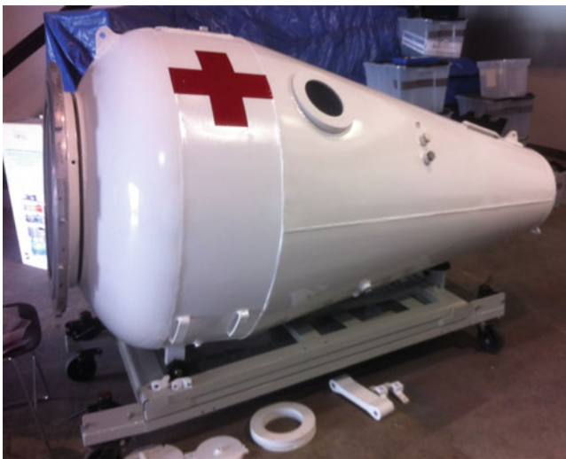
Fig. 42.21 An example of an EMS transport chamber which would admit the patient and paramedic in transport to a hospital-based unit from an event on the street; the ambulance would need no modification. Chamber would be powered by high-pressure D cylinders of compressed oxygen and air. The chamber would fit in the unmodified aisleway of a standard box compartment ambulance
