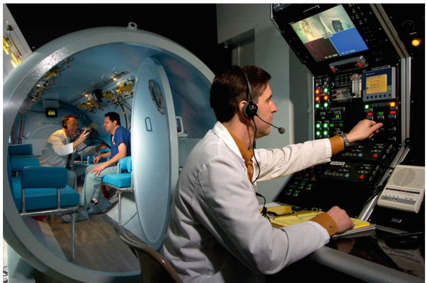
Fig. 7.7 (a) Large hyperbaric chamber at the University of Nagoya, Japan, outside view. (b) Inside view. Operations can be carried out in this chamber
