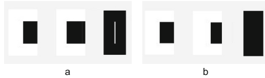
Fig. 2. (a) The left field of frame 17 and frame 18. We get the strong response in edge. (b) The left field of frame 17 and frame 16. There is no response at all.
