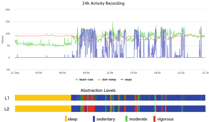
Fig. 3. Objective measurement and abstraction levels: on top you can see the first abstractions from accelerometer data: step counts together with heart rate and skin temperature measures. L1 and L2 show two abstraction levels for the activity recording.
