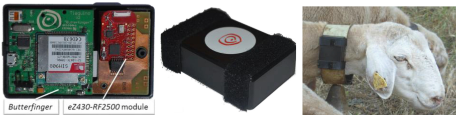
Fig. 3. The final version of the hardware, its protective case, and installation on a sheep collar.
