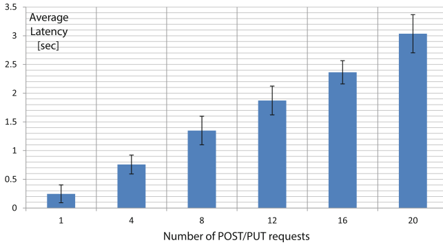
Fig. 5. Average latency for increasing number of POST/PUT requests (e.g. nodes). Also the standard deviation is denoted on the chart.
