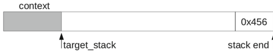
Fig. 2. Stack layout for a swapped out task. The saved context is on the top, target_stack points to the beginning of the saved control stack, and a fixed address, 0x456 , marks the bottom.
