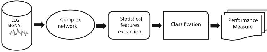
Fig. 1. The schematic diagram of proposed methodology for epileptic seizure detection.
