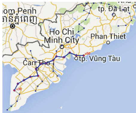
Fig. 12. The shortest path for data dissemination from node v_{50} to gateway node v_{36} . (Color figure online)
