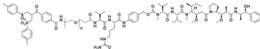
**Fig. 3.3** Example bis-sulphone reagent consisting of (*left to right*) a bis-sulphone linker, a PEG unit to aid solubility, an enzymatically cleavable self-immolative linker (valine-citrulline-*p*-aminobenzoyloxycarbonyl, *PAB*) and a cytotoxic payload (monomethyl auristatin E, *MMAE*). Reprinted with permission from *Mol. Pharmaceutics* 2015, 12, 1872–1879. Copyright 2015 American Chemical Society
