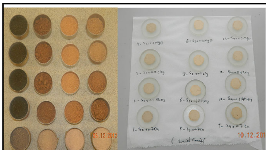
Fig. 7.14 Sample preparation procedures for XRD test
