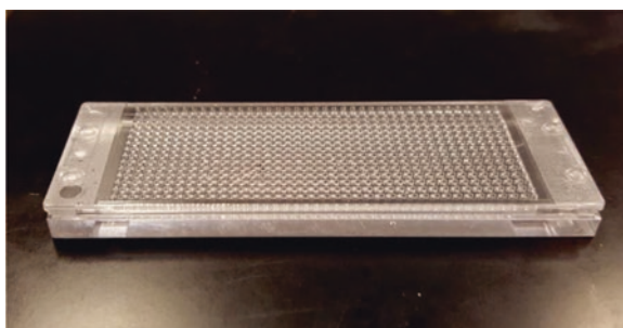
Fig. 4.9 Micropillar chip stamped on the shallow-well plate containing 500 μL of cold Matrigel-DPBS mixture
