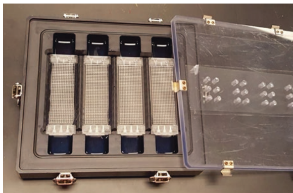
Fig. 4.7 Picture of a humid chamber with water. The lid will be put in place, and the chamber will be completely sealed to prevent water evaporation from growth medium in the microwell chip
