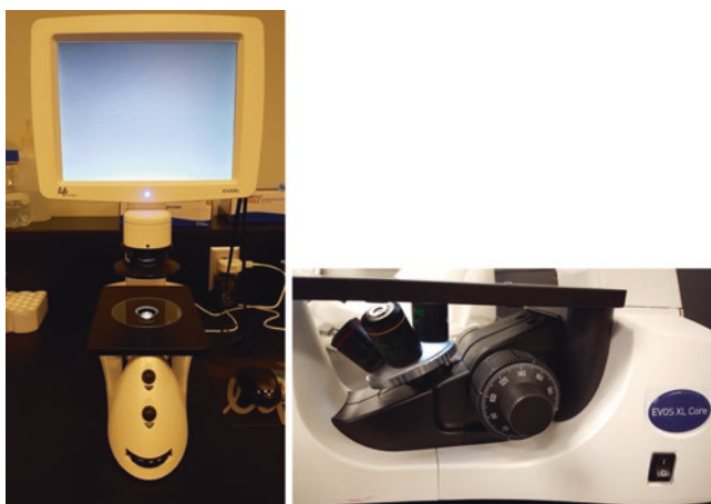
Fig. 4.12 Picture of the microscope with the on/off switch, objective lenses, and the focus adjustment knob: (Left) front view and (Right) side view
