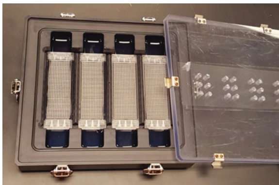
Fig. 3.14 Picture of a humid incubation chamber
