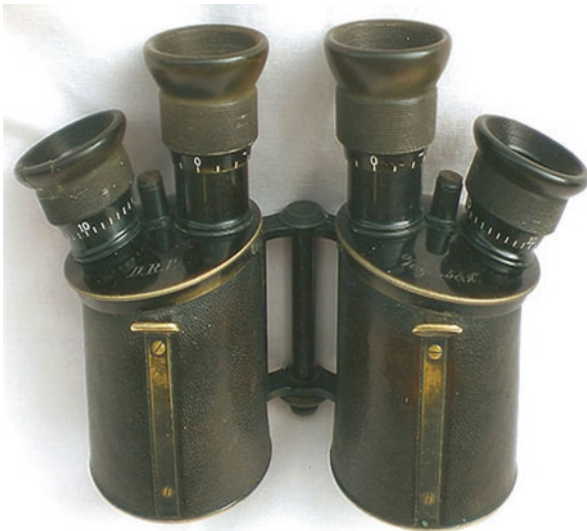
Fig. 3.42 A rare Carl Zeiss 5+10×24 mm “Marine-Glas m.Revolver” dual power turret binocular (circa 1896–1904). It was known as the “Admiral Togo Glass” because the commander of the Japanese in the Russo-Japanese war of 1904–1905 used this particular binocular. The construction of the body, objective lens cells and the method of securing the prisms are all similar to those used in the famous single power ‘Feldstecher’ binoculars. (Image credit: Antony Kay—OptRep— www.opticalrepairs.com )
