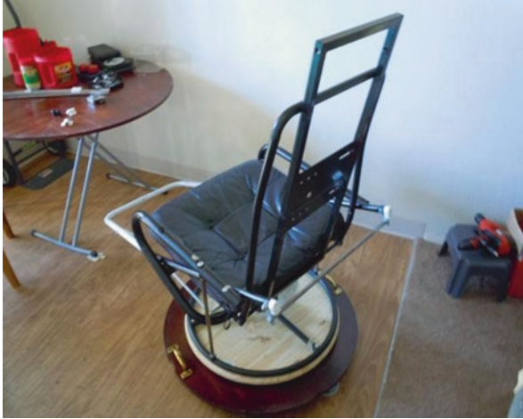
Fig. 3.31 The IKEA chair stripped down and ready to reassemble into a GOTO Binocular Chair (Image credit: Astronomy Technology Today)
