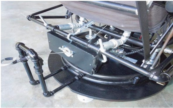
Fig. 3.33 The rear of the GOTO Binocular Chair with the altitude dual servomotor drive system in place (Image credit: Astronomy Technology Today)
