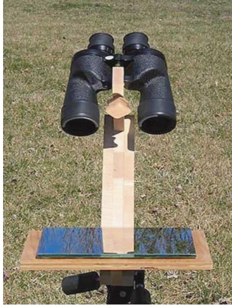
Fig. 3.15 This simple wooden binocular mirror mount setup looks good from all angles (Image credit: Rob Nabholz)
