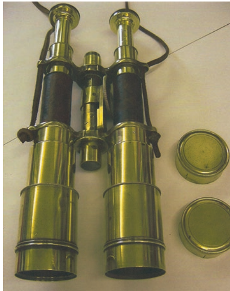
Fig. 3.5 A rare binocular telescope after restoration in the OptRep workshop. It was made by G&S Mertz (Munich) circa 1850 and its specification is 10x (approx.) with 35 mm air spaced objective lens, a rack, pinion eyepieces and telescopic eyepiece tubes. Fully extended, 11 in. in length. (Image credit: Antony Kay—OptRep— www.opticalrepairs.com )
