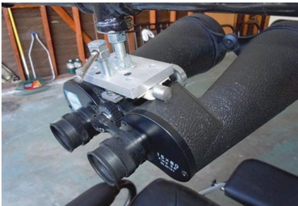
Fig. 3.34 The binocular mounting and adjusting system for the GOTO Binocular Chair (Image credit: Astronomy Technology Today)
