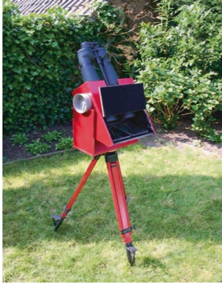
Fig. 3.11 Carl Vehmeyer made this splendid example of a binocular mirror mount. Notice the “trap door” for his binocular access to the sky (Image credit: Carl Vehmeyer)
