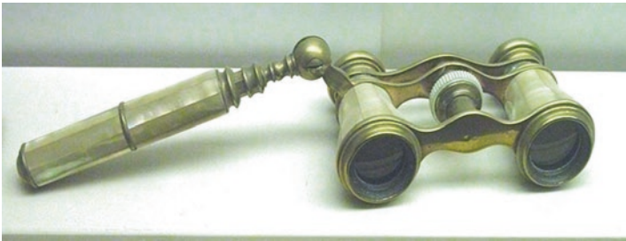
Fig. 3.46 Folding opera glasses made out of brass and Mother of Pearl (Image credit: Public Domain—Wikimedia Commons)
