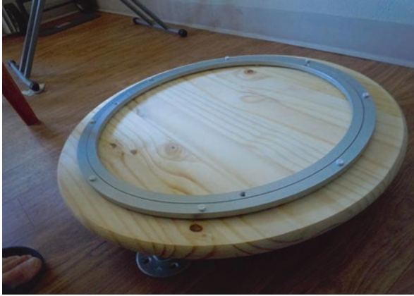
Fig. 3.30 The 17.5-in. dia. swivel bearing for the rotational base for the GOTO binocular chair (image credit: the Author)
