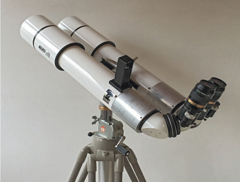
Fig. 10.28 Borg 125 mm Binoscope “2nd. edition cover image” with machined adapters and the dual eyepiece binback IPD adjustment system (Image credit: Jochen Schell— www.binoscopes.de )
