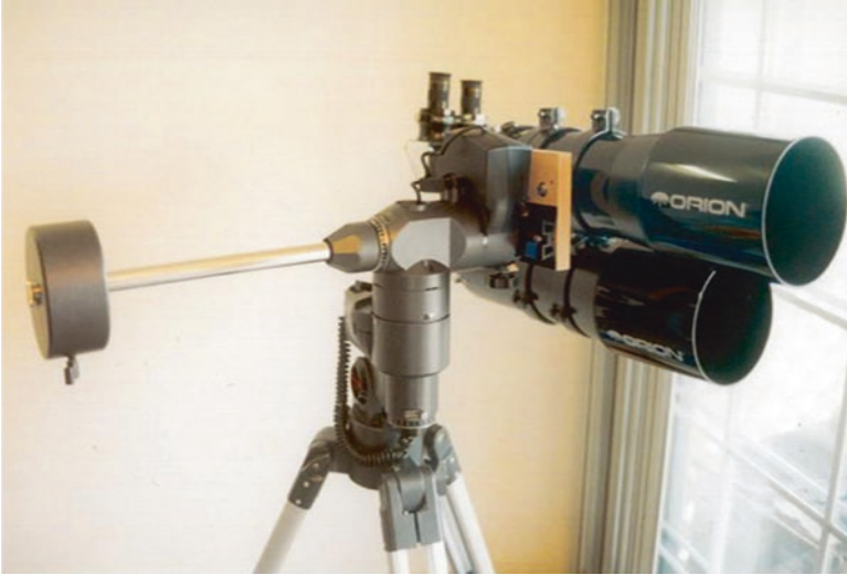
Fig. 10.17 The asymmetric 120-mm binocular telescope—front rear view (Image credit: Dr. Alex Tat-Sang Choy)
