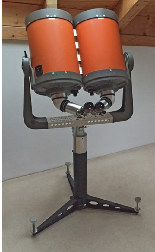
Fig. 10.22 Another view of the dual C-11's in their splendid Altazimuth mount (Image credit: Jochen Schell— www.binoscopes.de )
