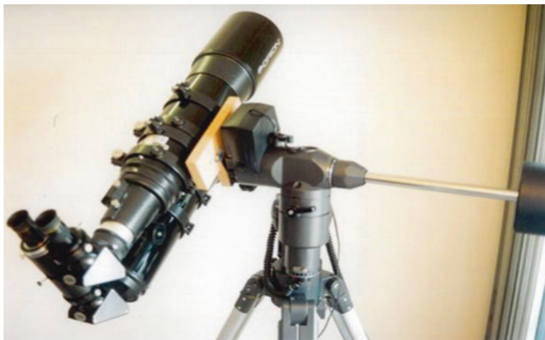
Fig. 10.18 The asymmetric 120-mm binocular telescope—rear view (Image credit: Dr. Alex Tat-Sang Choy)
