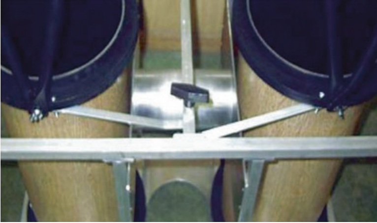
Fig. 10.13 The handle in the middle section rotates an arm that makes the two optical tubes swing apart via a pivot point. (Image credit: Wabash Valley Astronomical Society)
