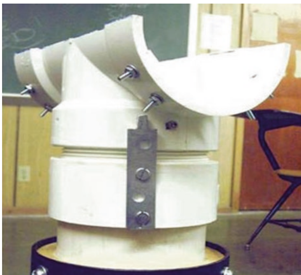
Fig. 10.11 PVC section sliced in half “T” that performs the heart of the mount (Image credit: Wabash Valley Astronomical Society)
