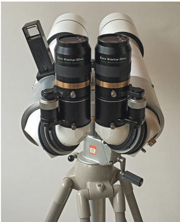
Fig. 10.27 Borg 125 mm Binoscope with the 2-inch dual 32 mm eyepiece binoback IPD adjustment system. Notice the interesting vertical dual aluminum knob focusing arrangement on each binoback (Image credit: Jochen Schell— www.binoscopes.de )
