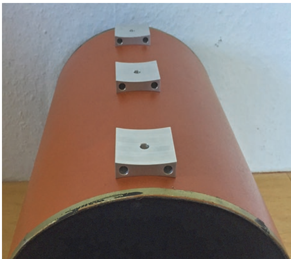
Fig. 10.24 Jochen used three equally spaced aluminum spacers that were machined to match the radius of the C-8 optical tube assemblies (Image credit: Jochen Schell— www.binoscopes.de )
