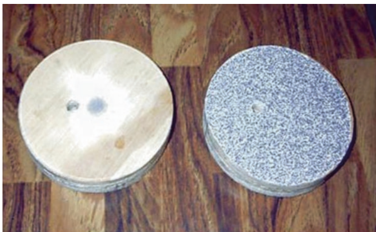
Fig. 10.12 Teflon pads were added to the “T” along with a stop (Image credit: Wabash Valley Astronomical Society)
