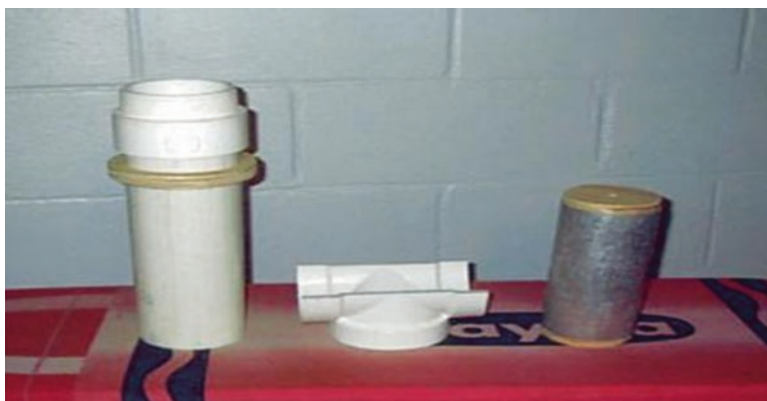
Fig. 10.9 The 4-in. PVC pipe section on the left that slides into the pier (Image credit: Wabash Valley Astronomical Society)
