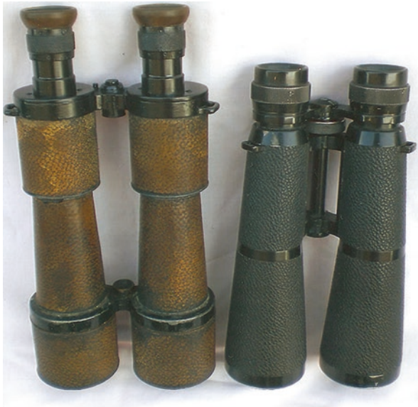
Fig. 3.6 A Carl Zeiss 10×50 mm (left) “Dekar” (circa 1950) and a Hensoldt (right) 10×50 mm “Dialyt” of post war vintage. Both are collectables (Image credit: Antony Kay—OptRep— www.opticalrepairs.com )
