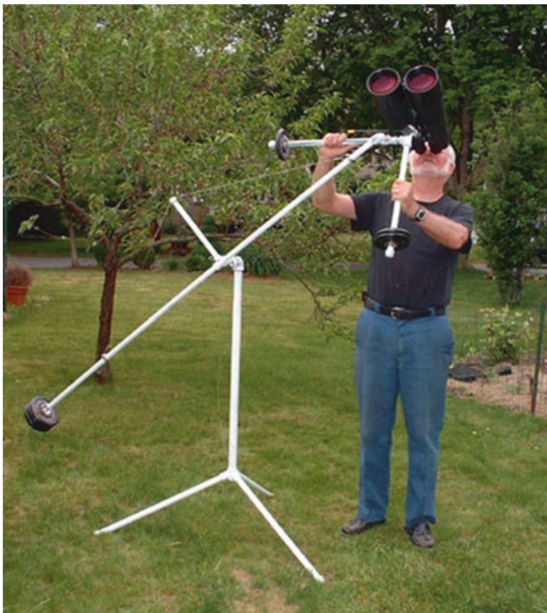
Fig. 5.41 An all pipe mount binocular stand. Sold as a kit called the “EZ Binoc Supermount” (Image credit: www.petersonengineering.com )
