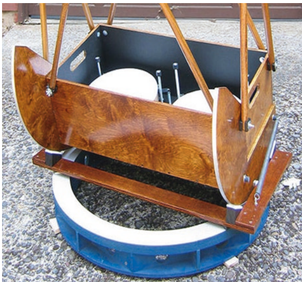
Fig. 5.75 The beautiful stained wood Altazimuth mount. This image still shows the Teflon pads (Image credit: Jerry Olton)
