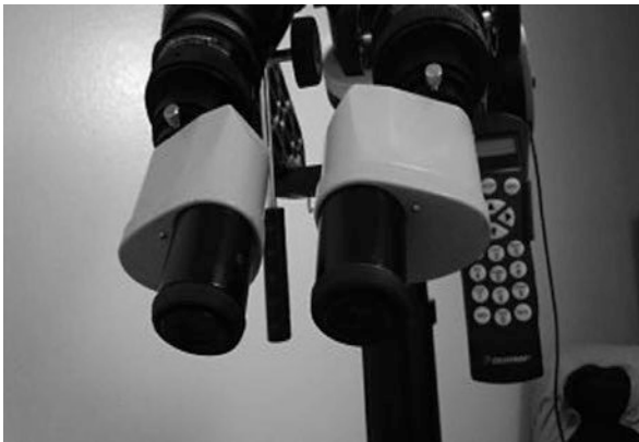
Fig. 2.21 How about a pair of 1¼-in. microscope eyepiece holders to use for a refractor binoscope? (Image credit: the Author)
