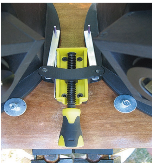
Fig. 5.74 Photo showing Jerry's very clever mechanical lead screw mechanism used for the IPD adjustment (Image credit: Jerry Oltion)
