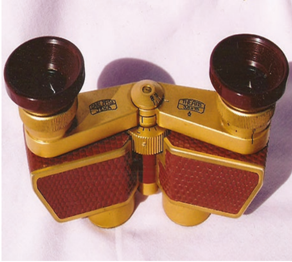
Fig. 3.45 A tiny Carl Zeiss 3.5×15 mm prismatic “pocket” binocular (Image credit: Antony Kay—OptRep— www.opticalrepairs.com )
