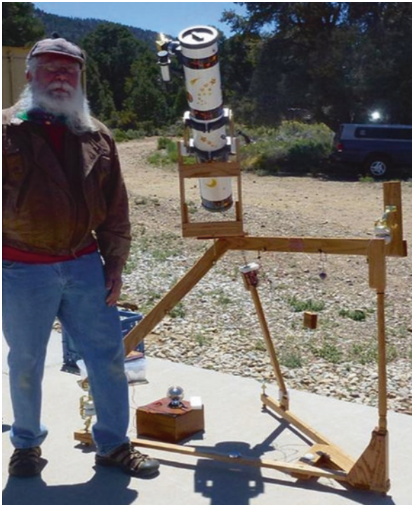
Fig. 4.21 Dann McCreary standing beside his homemade and quite unique 2012 RTMC merit award-winning “Pedagogical Equatorial Platform” (Image credit: Dann McCreary)
