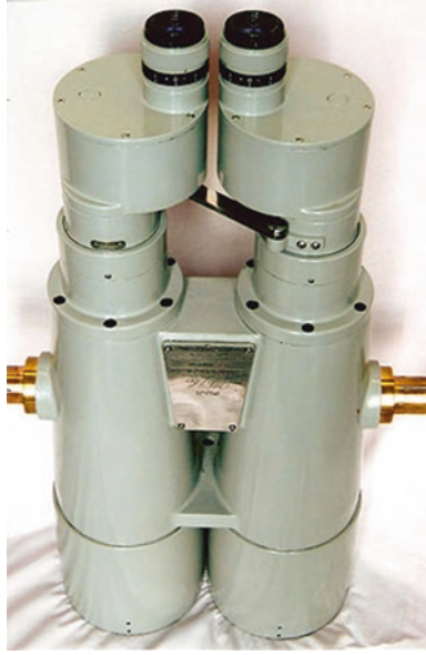
Fig. 3.8 A modern Fuji 40×150 mm “Meibo” binocular (Image credit: Antony Kay—OptRep— www.opticalrepairs.com )
