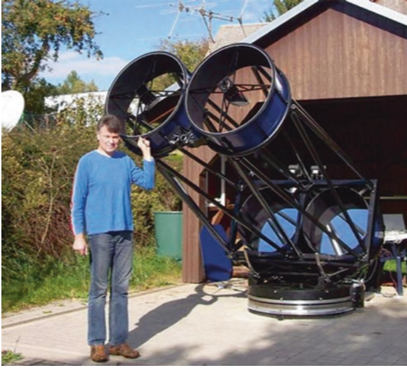
Fig. 5.3 Joerg Peter's 28" f/4.8 big binocular telescope certainly stands out in a crowd of telescopes at star parties (Image credit: Joerg Peters)
