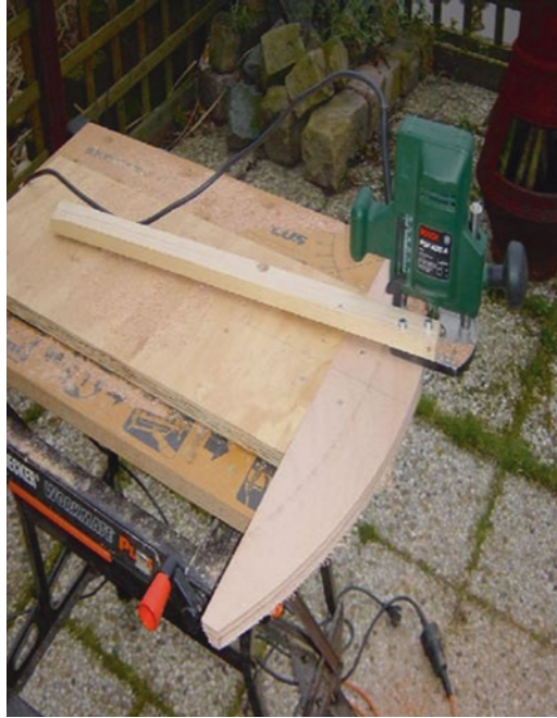
Fig. 8.2 Constructing the North sector bearing (Image credit: Andre Heijkoop)
