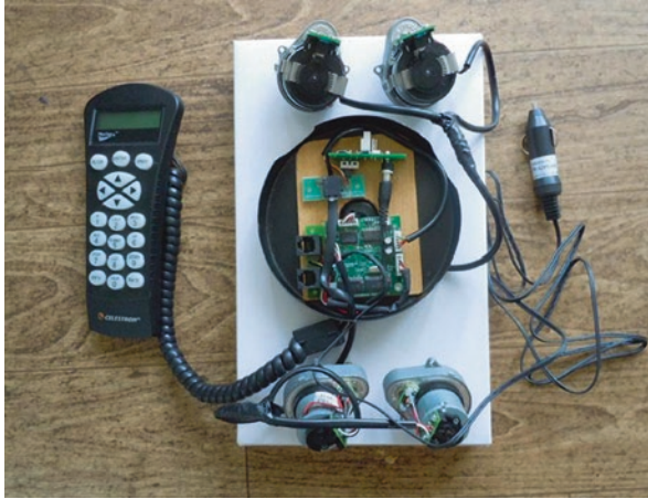
Fig. 3.35 NexStar 4SE electronics, servomotors, and controller for the GOTO Binocular Chair (Image credit: Astronomy Technology Today)
