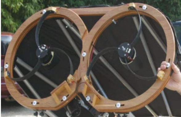
Fig. 2.14 Dave’s dual eyepiece IPD adjustment system for his 16 binocular telescope (Images credit: David Moorhouse)
