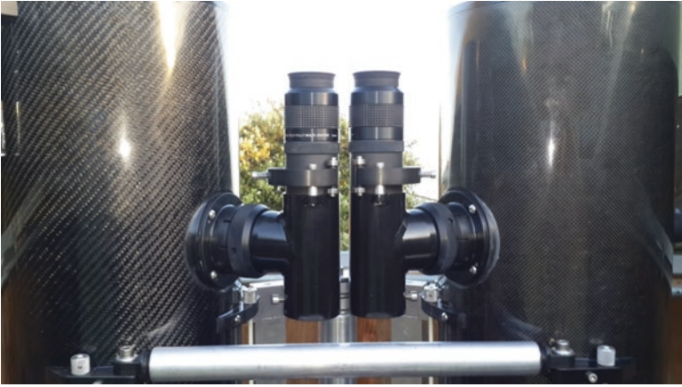
Fig. 7.38 Keith's binocular telescope tubes are made of carbon fiber. Check out his elegant dual eyepiece arrangement (Image credit: Keith Wilson)
