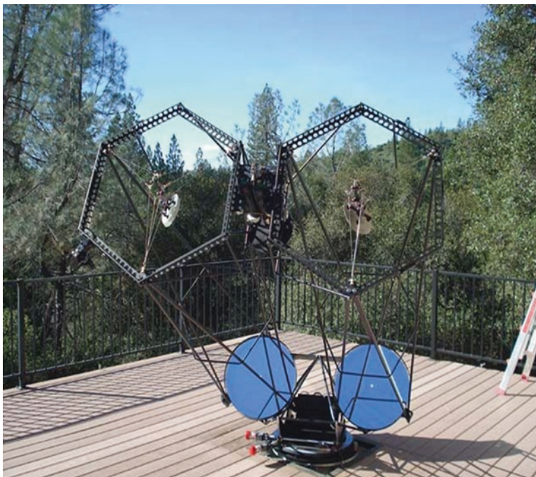
Fig. 5.65 Bruce Sayre's 22-in. splendid looking very open trust binocular telescope. See his personal comments on its performance from website ( http://brucesayre.net ) (Image credit: Bruce Sayre)
