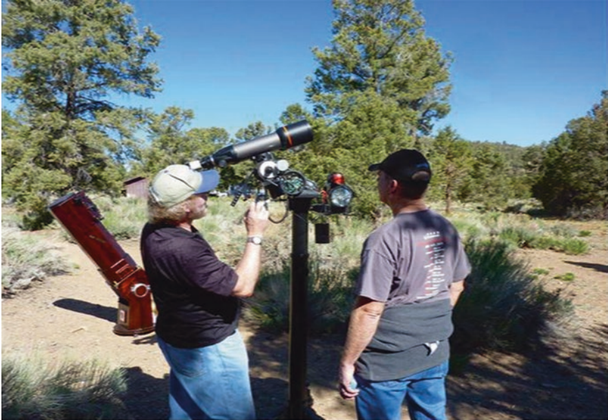
Fig. 6.6 Two RTMC amateur telescope makers discussing the author's homemade dual 102 mm f/6 GOTO Celestron binoscope at the 2011 RTMC (Image credit: Dann McCreary)
