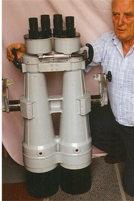
Fig. 3.2 Mr. Antony Kay and the 180 mm IJN binoculars, which have two-power eyepieces mounted on turrets that can be rotated to present the eyepieces for use. This binocular is 1.04 m (41 in.) long and weighs a hefty 64 kg (141 lb). Once serviced, this giant binocular was filled with nitrogen. (Image credit: Antony Kay—OptRep— www.opticalrepairs.com )
