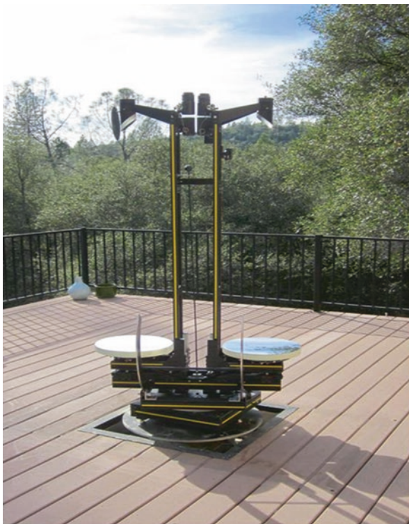
Fig. 5.6 Bruce Sayre's 14.5" elegant portable binoscope certainly demands attention at star parties (Image credit: Bruce Sayre)
