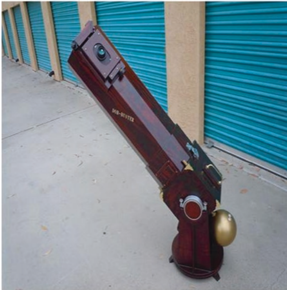
Fig. 6.14 The 10-in. f/4 “Dob Buster” with its 16-lb plus bowling ball counterweight (Image credit: the Author)
