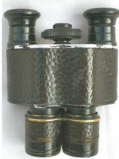
Fig. 3.4 A French inter-war binocular of unusual porro prism construction mounted on a flat plane. It has no IPD adjustment. (Image credit: Antony Kay—OptRep— www.opticalrepairs.com )
