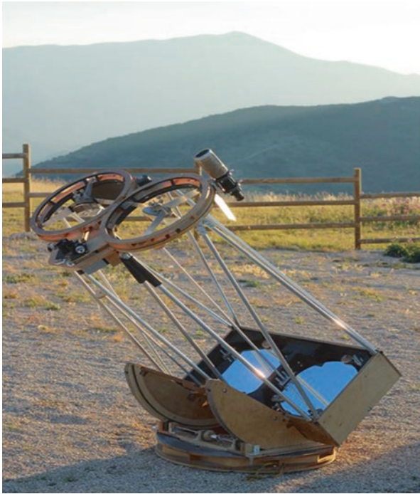
Fig. 5.61 Here's a photo of Eric Royer's big homemade 14-in. f/4.6 binocular telescope. Notice the rectangular box-shaped primary mirror section (Image credit: Eric Royer)
