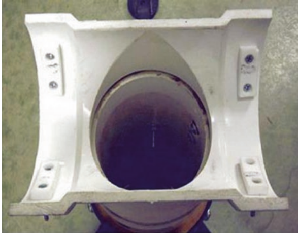
Fig. 10.10 PVC section sliced in half “T” that performs the heart of the mount (Image credit: Wabash Valley Astronomical Society)
