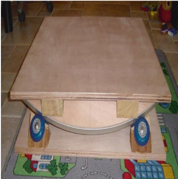
Fig. 8.3 For a perfect bearing surface, I used 30×2 mm aluminum (Image credit: Andre Heijkoop)
