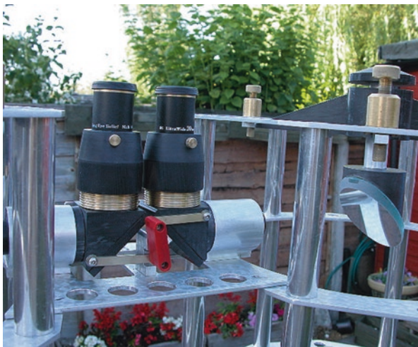
Fig. 2.4 Dual 2-in. eyepiece focusing system red lever IPD adjustment system on a 300 mm all-metal skeleton tube binocular telescope (Image credit: The Bolton Group— www.deep-sky.co.uk )
