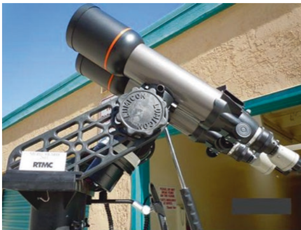
Fig. 6.2 Dual 102 mm f/6 Celestron GOTO binoscope on the Lumicon Universal Pier (Image credit: The Author)
