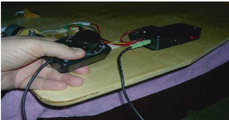
Fig. 8.20 Equatorial platform motor speed control unit (Image credit: Warren Philpot)
