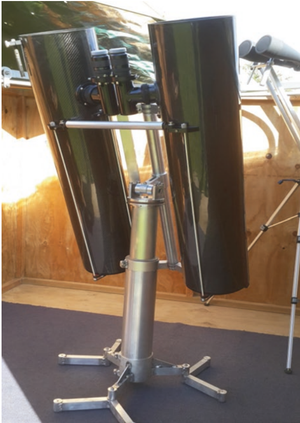
Fig. 7.39 An aluminum adjustable mount and pier setup with triangular-shaped tripod legs (Image credit: Keith Wilson)
