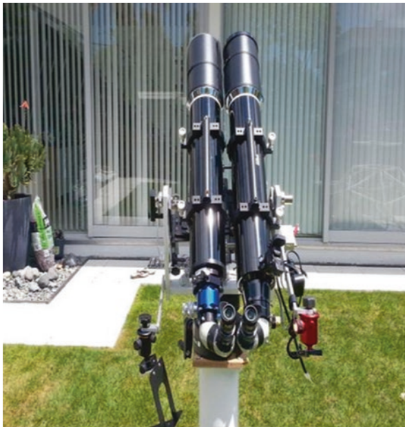
Fig. 5.13 Ian Gibbs has made an interesting dual 120 mm f/7.5 Equinox Sky Watcher ED refractor binoscope arrangement on a Altazimuth mounting. (Image credit: Ian Gibbs)
