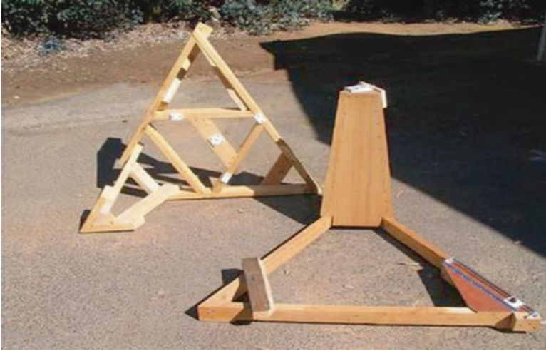
Fig. 8.28 The wooden base and the platform for the McCreary Mount (Image credit: Dann McCreary)
