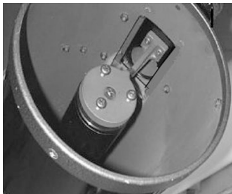
Fig. 2.9 A commercial single stalk secondary holder sled focuser on a Newtonian telescope (Image credit: the Author)
