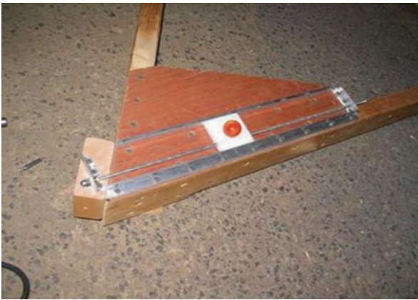
Fig. 8.32 This adjustment allows for a latitude range roughly between San Diego and Boston (32–42°) as well as “fine-tuning” the polar axis altitude (Image credit: Dann McCreary)
