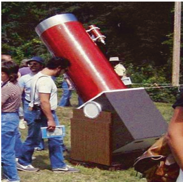
Fig. 1.1 A 1980s Dobsonian style Newtonian “rocker box” housed in an Altazimuth mount (Image credit: Halfblue-Wikimedia Commons)
