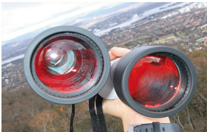
Fig. 7.34 Binoculars with red colored multi-coated objective lenses (Image credit: Dfrg.msc—CC BY-SA 3.0—Wikimedia Commons)
