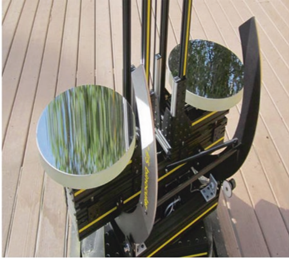
Fig. 5.7 Here's another closer look at Bruce Sayre's portable binocular telescope's 14.5-in. dual primary mirror cell support system (Image credit: Bruce Sayre)
