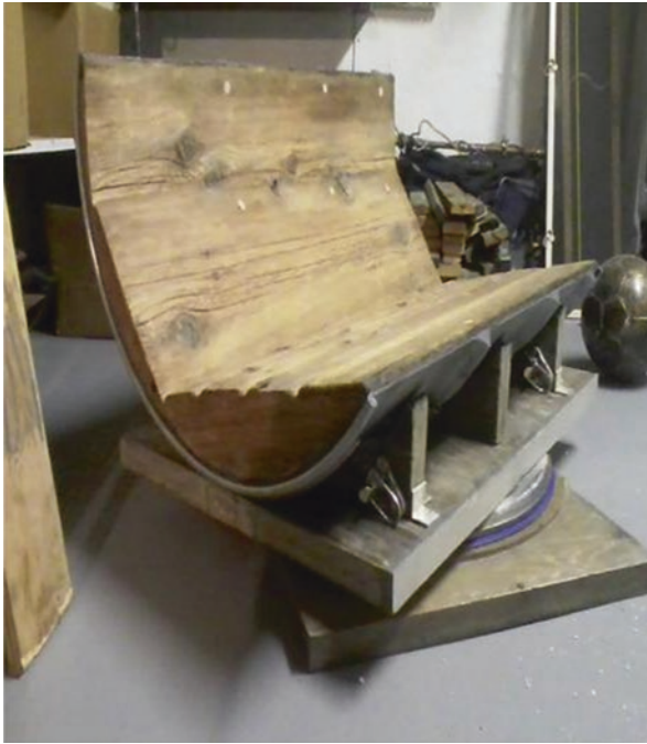
Fig. 5.57 This photo shows the cutaway section of the 55-gal oil drum on the rotating Altazimuth base that makes up the primary mirror cell support for Doug's 12.5-in. binocular telescope (Image credit: Doug Chapman)
