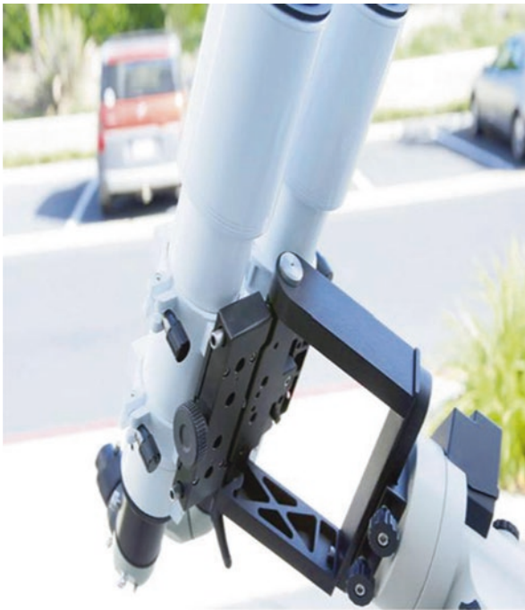
Fig. 5.29 Hutech offers a nice equatorial AOK platform that is mounted axially between the forks, providing the observer a way to adjust for good head and eye position as the binoscope moves equatorially across the night sky (Image credit: Borg/Hutech)
