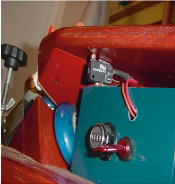
10 revolutions linear pot with digital readout
