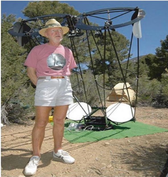
Fig. 5.8 Bruce Sayre's very open truss 22-in. giant binocular telescope won a merit award at the 2004 RTMC (Image credit: Robert Stephens RTMC)
