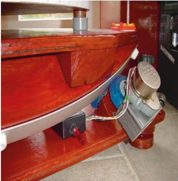
Fig. 8.7 I replaced the little black box with a bigger blue box with all the electronics in it (Image credit: Andre Heijkoop)
