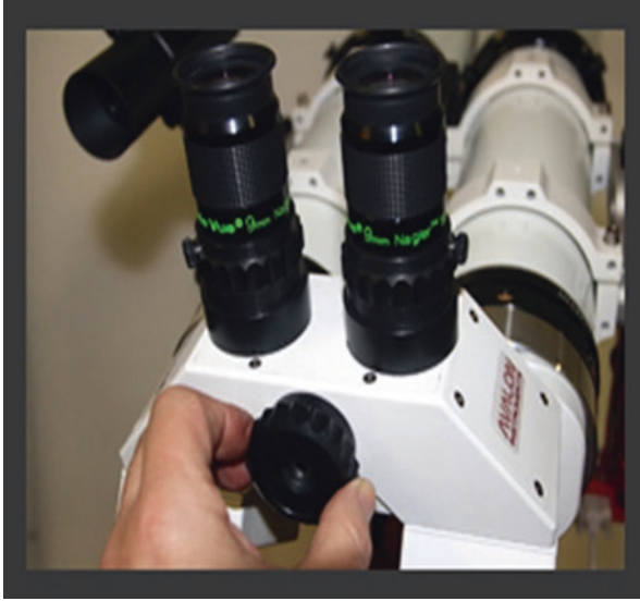
Fig. 5.68 The IPD adjustment is easily made with just a twist of the knob. Eyepieces are independently focused (Image credit: www.avalon-instruments.com )
