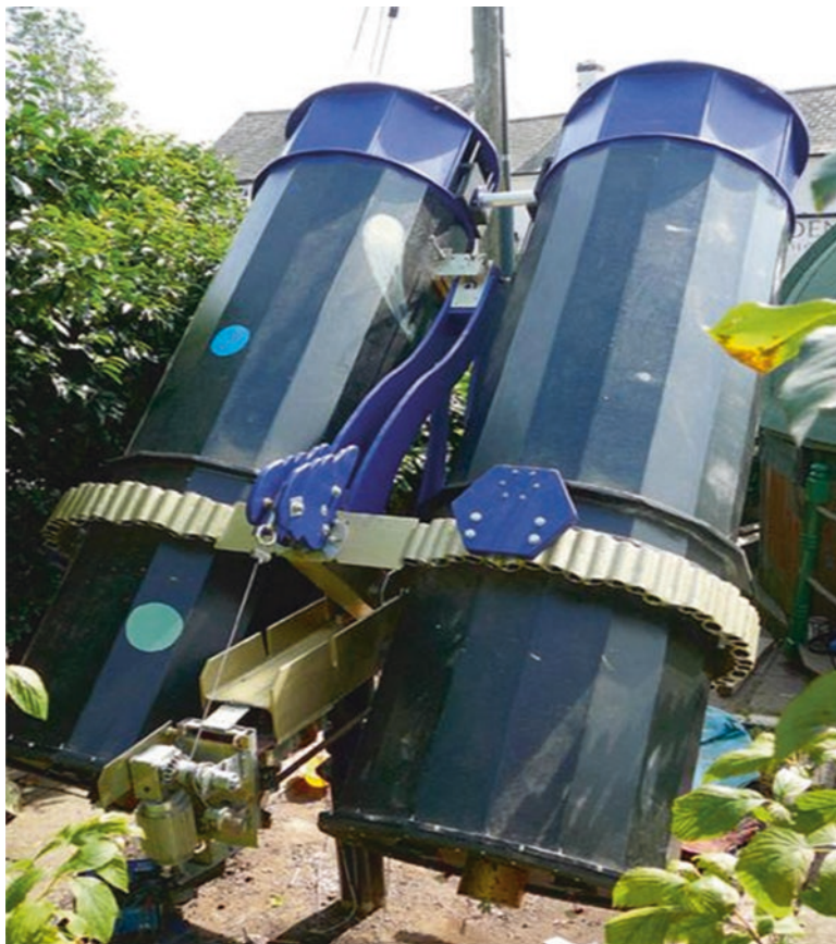
Fig. 5.45 Call it “Hexy”. Here’s a rear view of the big 16.1-in. f/4.7 binocular telescope (Image credit: Danny Strong)
