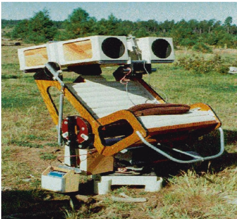
Fig. 5.15 Pierre Schwarr made this motorized with two homemade 8-in. f/4 binocular telescopes mounted on top (Image credit: Steve Dodder)
