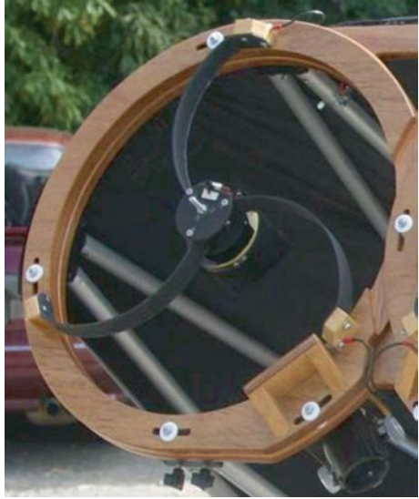
Fig. 2.17 Dave’s curved spider vane holder system for his 16-in. binocular telescope (Image credit: David Moorhouse)
