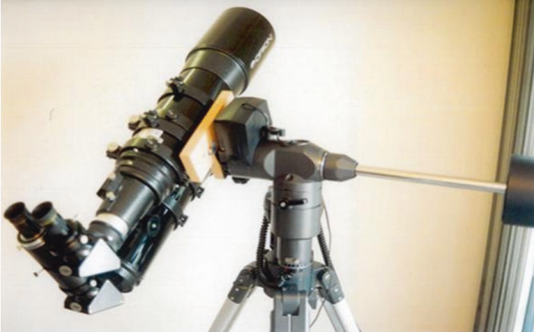
Fig. 10.18 The asymmetric 120-mm binocular telescope—rear view (Image credit: Dr. Alex Tat-Sang Choy)
