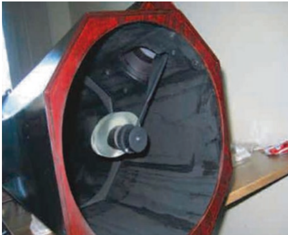
Fig. 6.16 The Dob Buster single stalk secondary mirror holder (Image credit: the Author)
