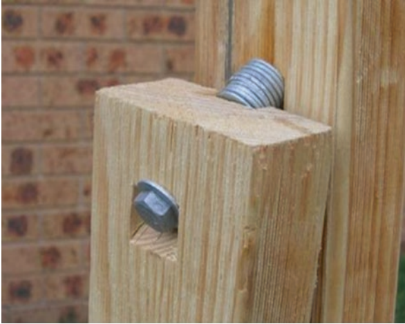
Fig. 8.25 The equatorial cradle showing the top polar pivot end (Image credit: Chris Luton)
