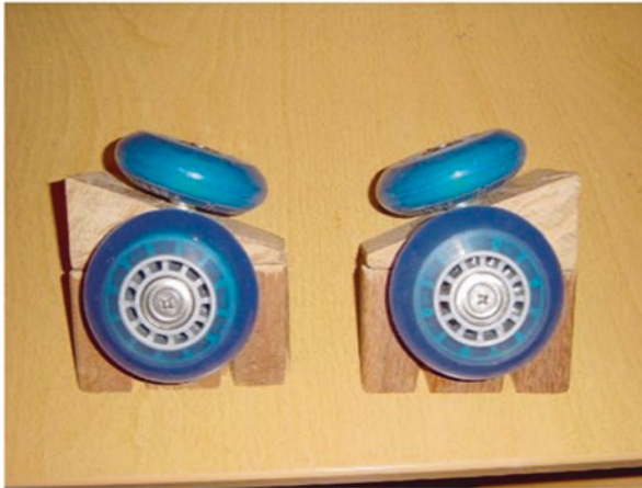
The North Bearing Supports
