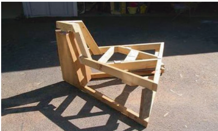
Fig. 8.29 The platform resting on the base of the McCreary Mount (Image credit: Dann McCreary)
