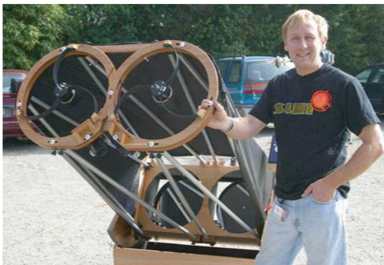
Fig. 5.25 David Moorhouse of New Zealand proudly shows off his elegant homemade wooden 16-in. truss tube binocular telescope (Image credit: David Moorhouse)
