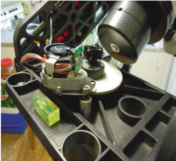
Fig. 6.3 The azimuth gear and knob and clutch system (Image credit: the Author)
