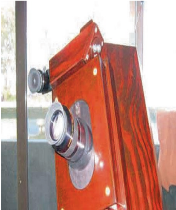
Fig. 7.25 A “Periscope-Style” right-angle 30-mm finder on the 10’ f/4 homemade “Dob Buster” Newtonian telescope (Image credit: The Author)
