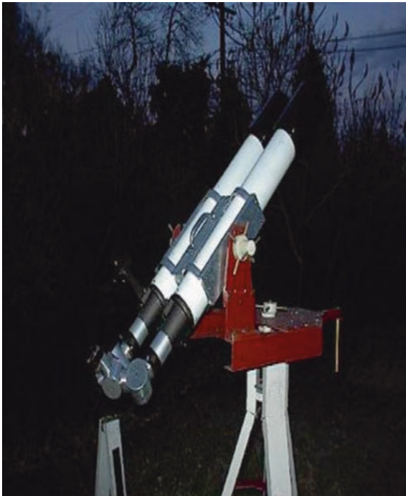
Fig. 5.10 Dave Trott made this nice looking 4-in. f/10 refractor binoscope combined with a pair of homemade binobacks on a simple Altazimuth mount (Image credit: Dave Trott)
