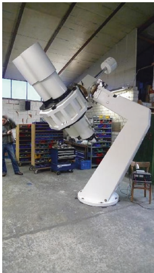
Fig. 5.31 A front view of APM's big custom looking 12-in. f/7.5 triplet APO refractor binoscope on it's computer controlled mount (Image Credit: Marcus Ludes— www.apm-telescopes.de )
