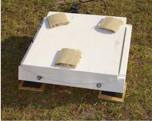
Fig. 8.38 Michael Davis's equatorial platform for his big 17.5-in. Dobsonian telescope (Image credit: Michael Davis)
