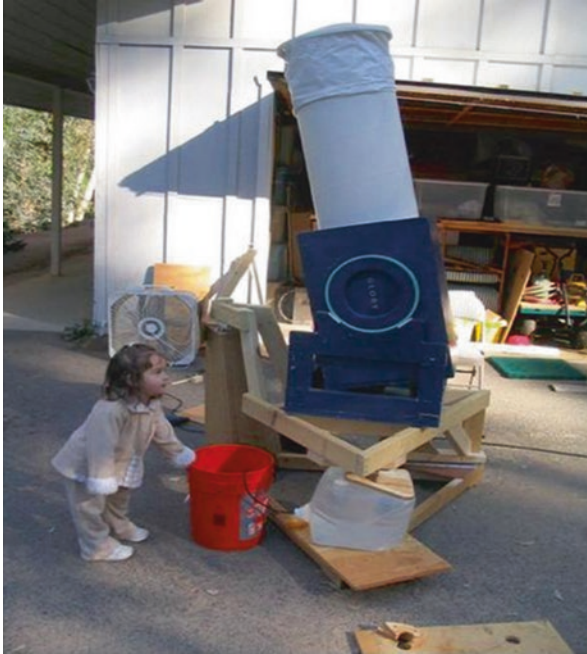
Fig. 8.35 The McCreary Mount with a Dobsonian installed on top of the platform with assistant (Image credit: Dann McCreary)
