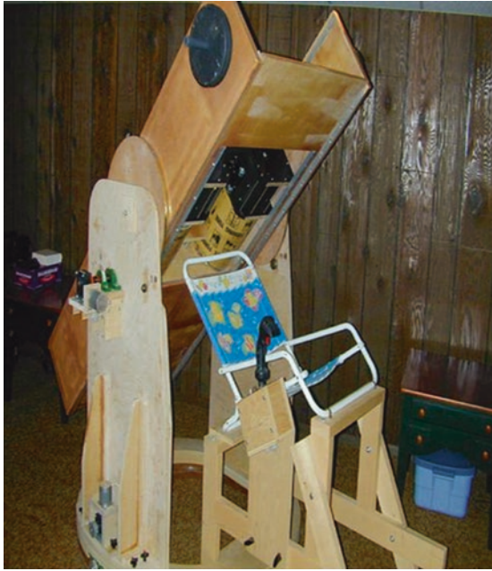
Fig. 5.50 Ray Jurevicius designed and built this splendid looking 8-in. f/6 all-wood binocular telescope that has a lawn chair mounted on top of the bottom section of the Altazimuth mount (Image credit: Ray Jurevicius)
