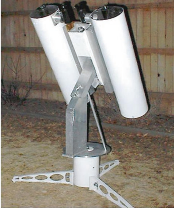
Fig. 5.54 Here is the lower section view of Dave Trott's all-aluminum 6-in. binocular telescope showing the binocular telescope tube support system along with the Altazimuth mounting with the pier and tripod legs (Image credit: Dave Trott)
