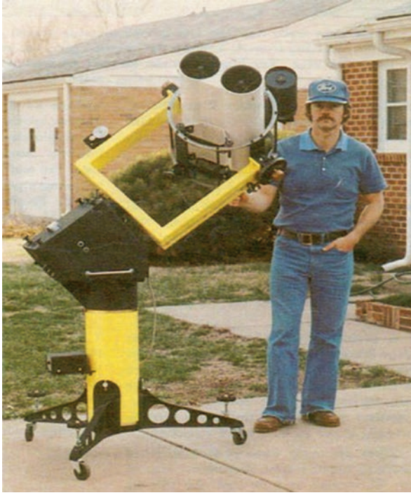
Fig. 6.8 The author with his homemade dual 6-in. f/15 Dall-Kirkham Cassegrain binoculars won the Engineering Merit Award at the 1981 (RTMC) Riverside Telescope Makers Conference (Image credit: Rick Schmidt)
