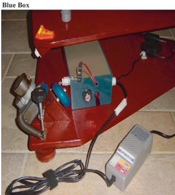
Fig. 8.8 The blue box contains the electronics to drive the Stepper Motor (Image credit: Andre Heijkoop)
