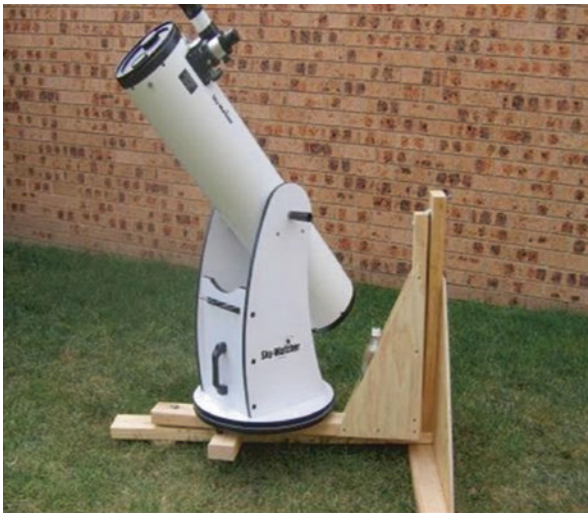
Fig. 8.24 The equatorial cradle can reach any part of the sky dome (Image credit: Chris Luton)
