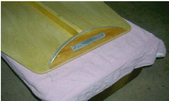
Fig. 8.16 Equatorial platform rear bearing support (Image credit: Warren Philpot)
