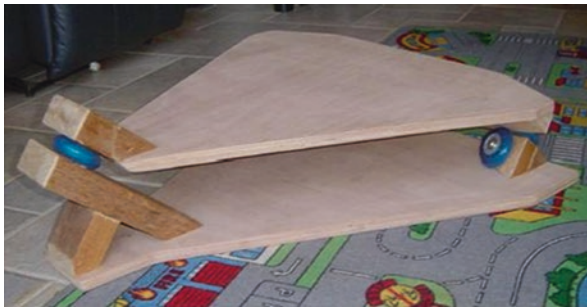
Fig. 8.5 I also used an inline skate wheel for the South bearing (Image credit: Andre Heijkoop)
