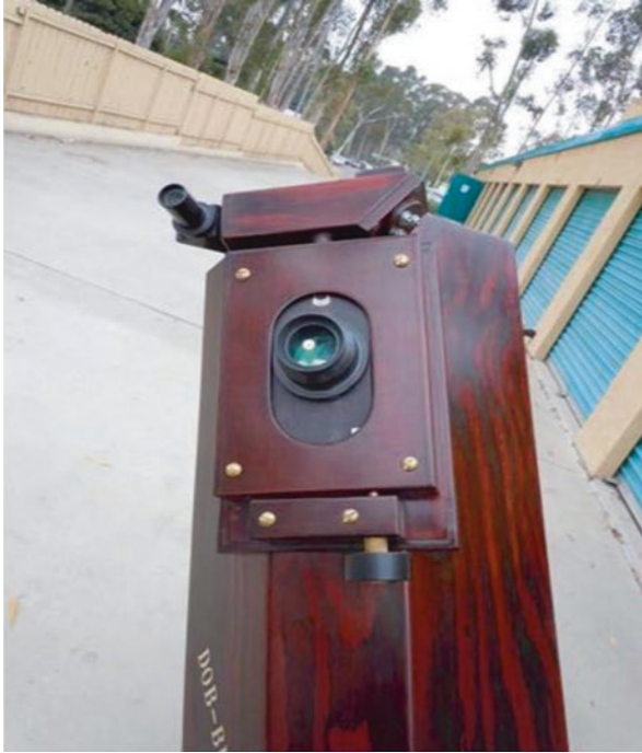
Fig. 6.15 The Dob Buster “sled” focuser (Image credit: the Author)
