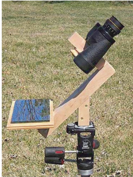
Fig. 3.14 A very nice, stable binocular mirror mount with a simple design (Image credit: Rob Nobholtz)
