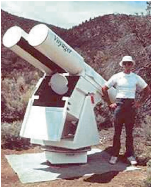
Fig. 3.18 Wayne Schmidt standing next to his motorized 8-in. f/8 binocular telescope at the 1995 RTMC (Image credit: Robert Stephens—RTMC)
