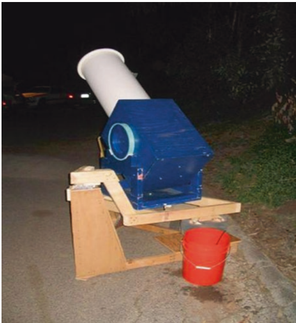
Fig. 8.27 The McCreary Mount with a Dobsonian telescope sitting on the equatorial platform (Image credit: Dann McCreary)
