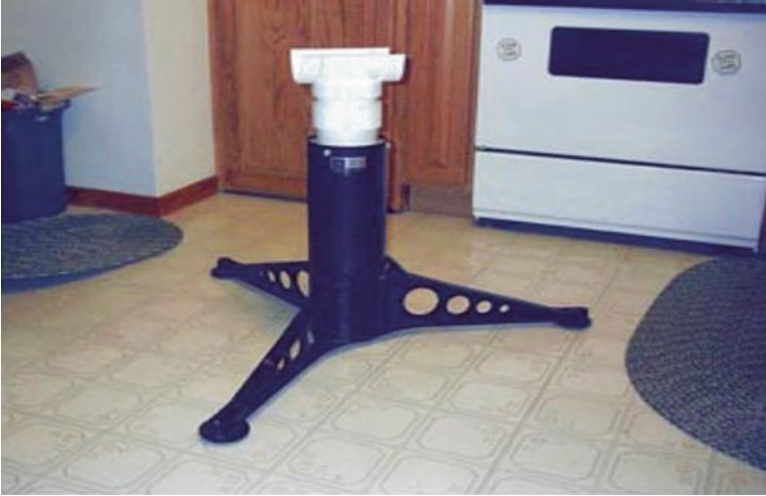
Fig. 10.14 The 8-in. binocular telescope pier with altitude bearing attached (Image credit: Wabash Valley Astronomical Society)
