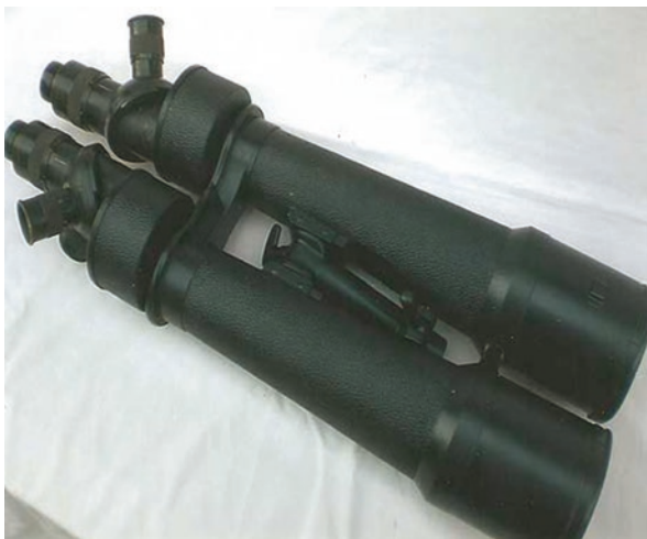
Fig. 3.43 A Carl Zeiss 12–20–40×80 mm turret binoculars (Asembi) was used in WW1 and WW2 by the Kriegs marine. The design remained unchanged with one of the few changes being that the air-spaced objective lenses were eventually replaced with cemented ones in the later models. The prism housings can be swiveled to change the IPD and also be swung outwards to allow two observers to use it as two separate telescopes observing the same target. (Image credit: Antony Kay—OptRep— www.opticalrepairs.com )
