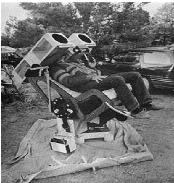
Fig. 5.18 Pierre Schwarr and his dual 8-in. f/4 Newtonian binocular telescope motorized chair (Image credit: Robert Stephens RTMC)
