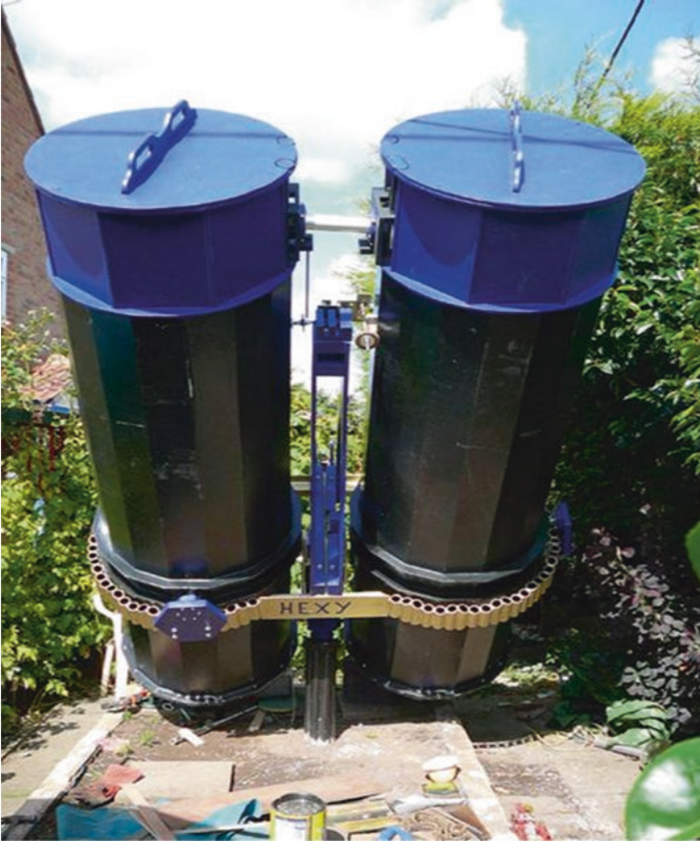
Fig. 5.44 Danny Strong of the UK has made this very impressive 16.1-in. f/4.7 Goliath of a binocular telescope (Image credit: Danny Strong)
