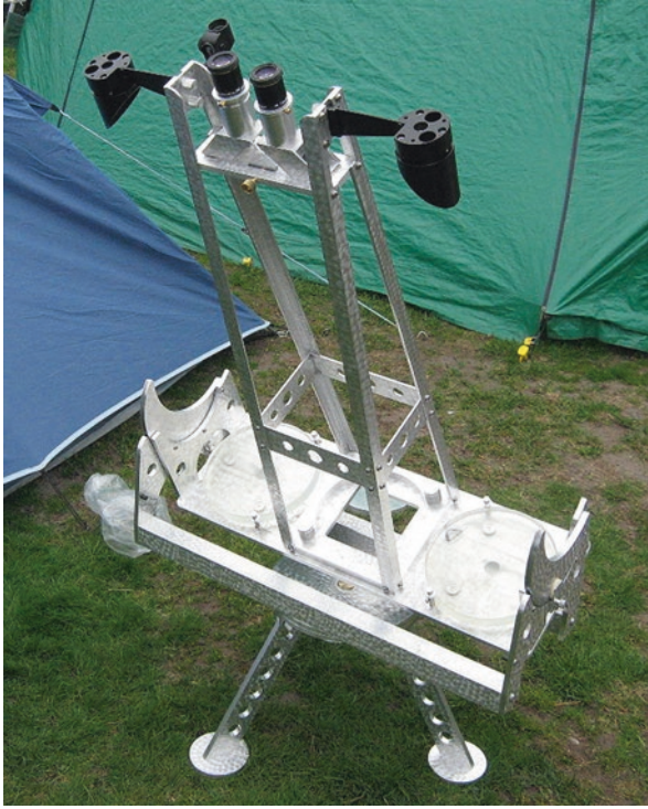
Fig. 10.38 They're almost finished with the exception of the un-coated mirrors....It's almost ready to start pumping photons through those dual eyepieces. (Image credit: www.deep-sky.co.uk )
