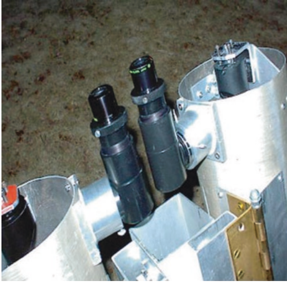
Fig. 2.12 Dave Trott designed this clever hinged dual 6-in. binocular telescope that is similar to a basic pair of binoculars (Image credit: Dave Trott)
