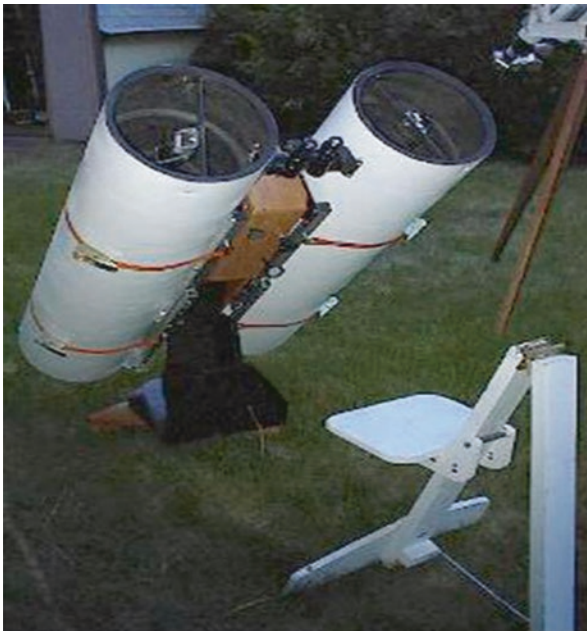
Fig. 5.11 Here's another example of Dave's handy work, a 13.1-in. Sonotube binocular telescope (Image credit: Dave Trott)
