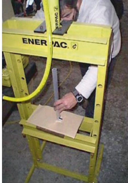
Fig. 10.6 The fitting being pressed into a tube section (Image credit: Wabash Valley Astronomical Society)
