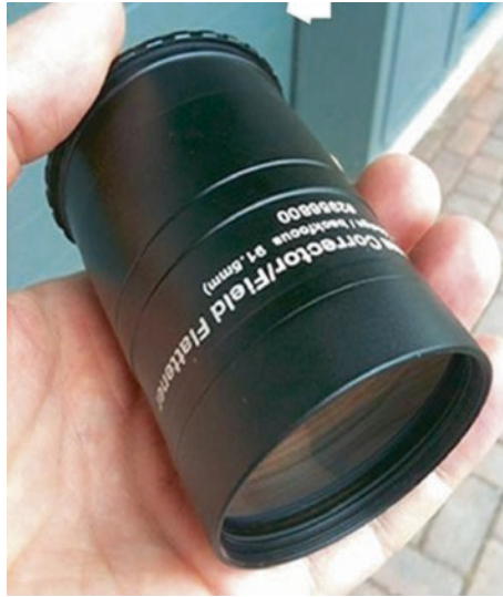
Fig. 2.3 Baader Rowe Coma Corrector and field flattener (Image credit: First Light Optics)
