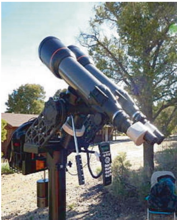
Fig. 6.1 2011 RTMC Warren Estes Memorial Award winning Dual 102 mm f/6 Celestron GOTO binoscope (Image credit: the Author)
