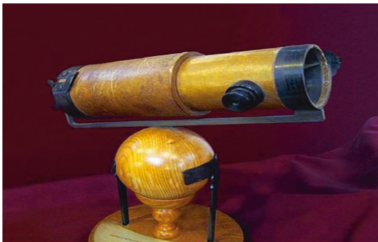
Fig. 4.13 A replica of the original Newtonian reflector (Image credit: Solipsist/Andrew Dunn-Wikimedia Commons)
