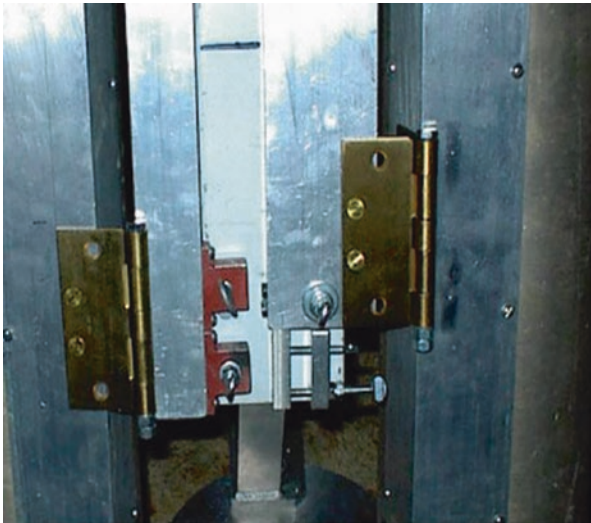
Fig. 2.13 Pictured are the push/pull bolts for vertical (on the left ) and horizontal (on the right ) IPD adjustment (Image credit: Dave Trott)
