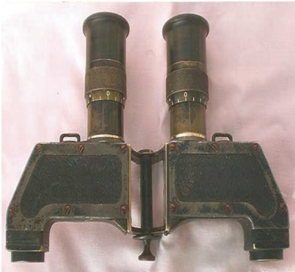
Fig. 3.3 Here is an example of a Carl Zeiss 3×20 mm Teleplast (Circa: 1907–1911) It has Sprenger prisms and triple element field lens. (Image credit: Antony Kay—OptRep— www.opticalrepairs.com )
