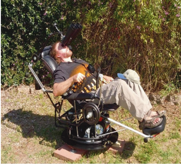
Fig. 3.28 The author's homemade GOTO servomotor-powered binocular chair (Image credit: the Author)
