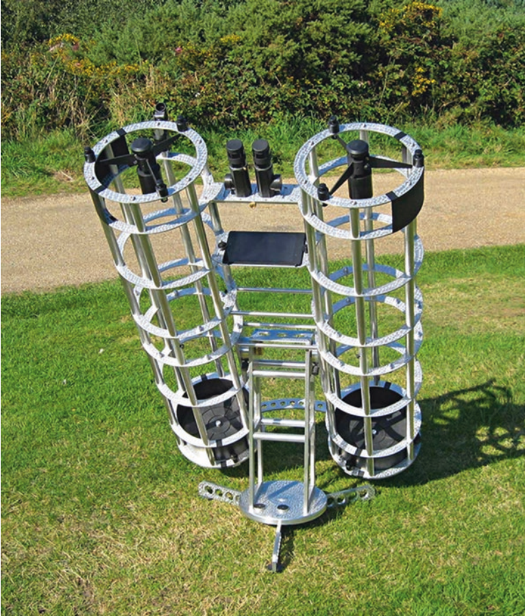
Fig. 5.19 A dual 200 mm (7.87 in.) nicely machined open tube binocular telescope (Image credit: David Ratledge—The Bolton Group— www.deep-sky.co.uk )
