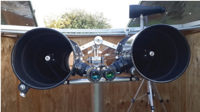
Fig. 7.37 Looking down the business end of Keith Wilson's splendid looking dual homemade 10-in. binocular telescope (Image credit: Keith Wilson)
