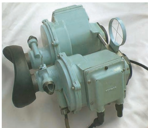
Fig. 3.44 A British AVIMO warship binocular, type G389/1 fitted with electrical heaters and internal filters. These binoculars, which have many unusual features along with the smaller G386/3, were the last types designed by AVIMO before the company was drawn in by Thales. This type of binocular is used by the Royal Navy and the navies of many other countries. (Image credit: Antony Kay—OptRep— www.opticalrepairs.com )
