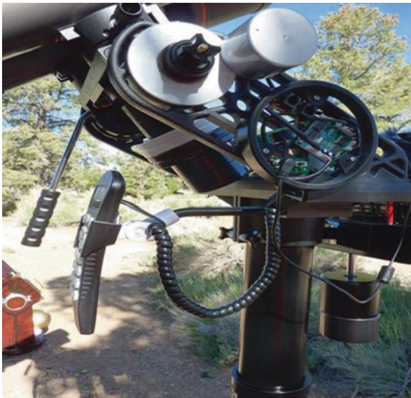
Fig. 6.7 The side view of the dual 102-mm GOTO Celestron binoscope showing the altitude drive gear, electronics package, hand controller, and counterweight system (Image credit: Dann McCreary)
