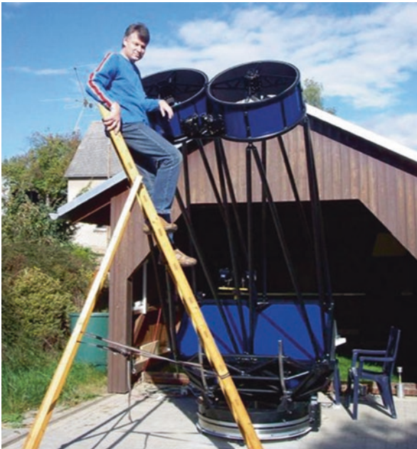
Fig. 5.4 Joerg's big 28" binocular telescope is the current largest ATM binocular telescope around (Image credit: Joerg Peters)
