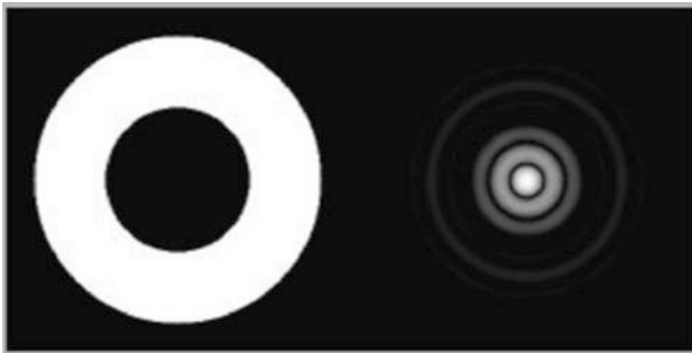
Fig. 1.18 Fifty percent central obstruction and the resulting diffraction pattern (Image credit: Rene Pascal)
