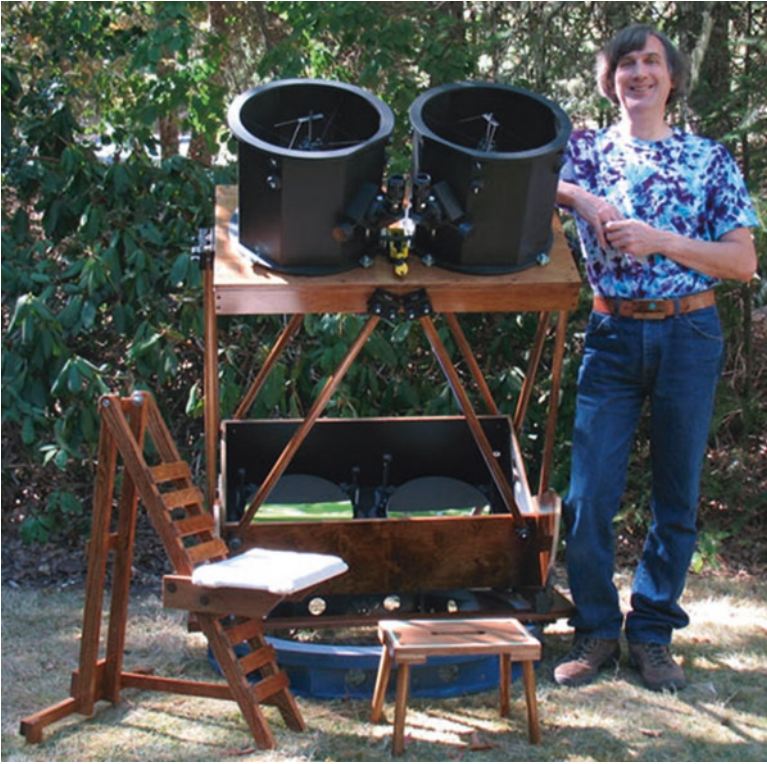
Fig. 5.70 Jerry Olton with his homemade dual 12.5 in. f/4.6 Dobsonian style binocular telescope (Image credit: Jerry Olton)
