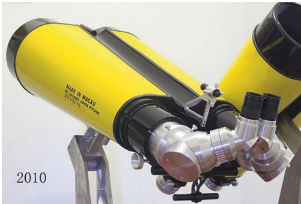
Fig. 3.47 A splendid looking giant pair of homemade 203 mm giant binoculars (Image credit: Luciano Jorge Ritchie of Macau)
