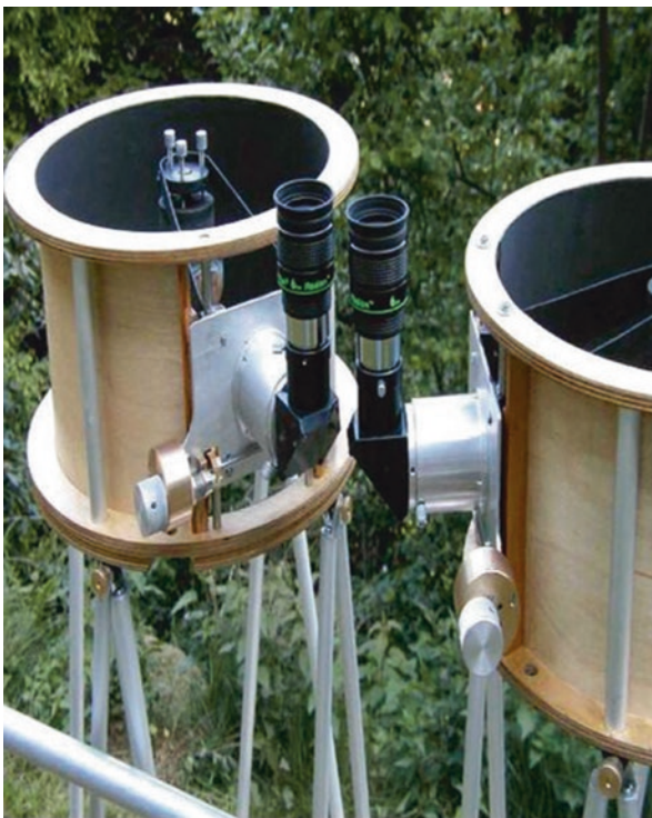
Fig. 5.23 Ulrich Vedder's beautifully machined dual eyepiece focuser system complete with two big Televue eyepieces (Image credit: Ulrich Vedder)
