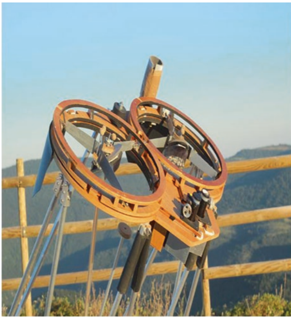
Fig. 5.62 Another view of Eric Royer's splendidly crafted open tube truss binocular telescope. Note the secondaries and their support system along with his dual reverse focuser arrangement mounted in a secure fashion in the solid dual wooden rings (Image credit: Eric Royer)
