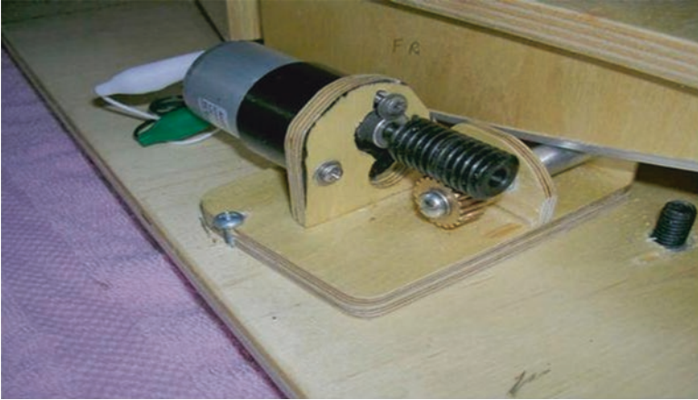
Fig. 8.18 Equatorial platform drive assembly (Image credit: Warren Philpot)
