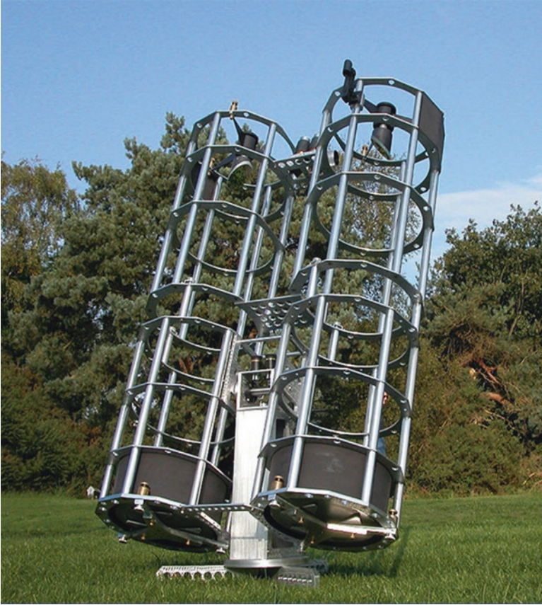
Fig. 5.42 A dual 300 mm (11.8 in.) binocular telescope with a splendidly machined skeleton tube system (Image credit: David Ratledge—The Bolton Group— www.deep-sky.co.uk/telescopemaking.htm )
