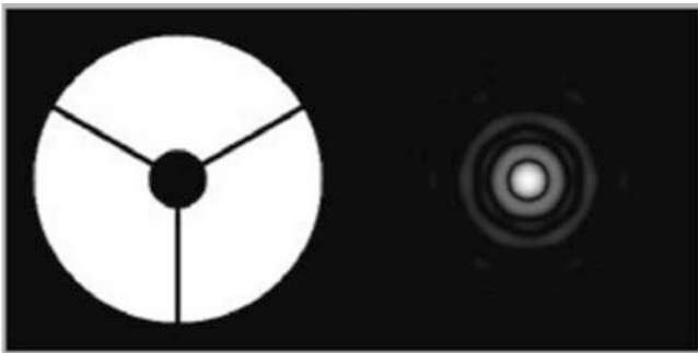
Fig. 1.20 A three-vane spider that is 1.55 of the diameter of the main mirror thick, combined with a central obstruction of 20% (Image credit: Rene Pascal)
