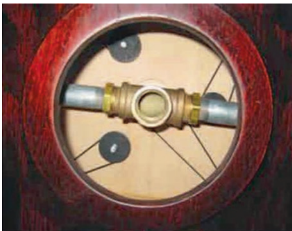
Fig. 6.17 The “Dob Buster” O-ring combination wooden pulley collimation system with the bowling ball counterweight shaft mounting flange in the center (Image credit: the Author)
