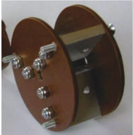
Fig. 2.18 Dave’s three curve vain holder system for his 16-in. binocular telescope (Image credit: David Moorhouse)
