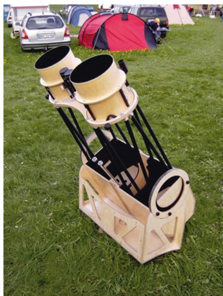
Fig. 2.23 A nice example of a homemade Dobsonian binocular telescope (Image credit: ECeDee—Wikimedia Commons)
