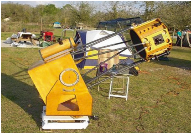
Fig. 8.36 Michael Davis’s big 17.5-in. Dob sits on his newly constructed equatorial platform (Image credit: Michael Davis)
