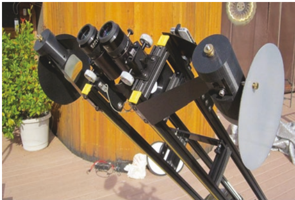
Fig. 2.7 Bruce Sayre's elegant 14.5 portable binocular telescope has a simple IPD feature (Image credit: Bruce Sayre)
