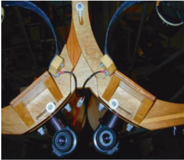
Fig. 2.16 Dave’s dual eyepiece IPD adjustment system for his 16 binocular telescope showing the dual eyepieces adjusted “out” (Image credit: David Moorhouse)
