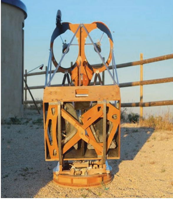
Fig. 5.63 The rear section of Eric's big binocular telescope showing the 14-in. f/4.6 aluminum primary mirror cell support system, a very interesting mirror cell design indeed (Image credit: Eric Royer)
