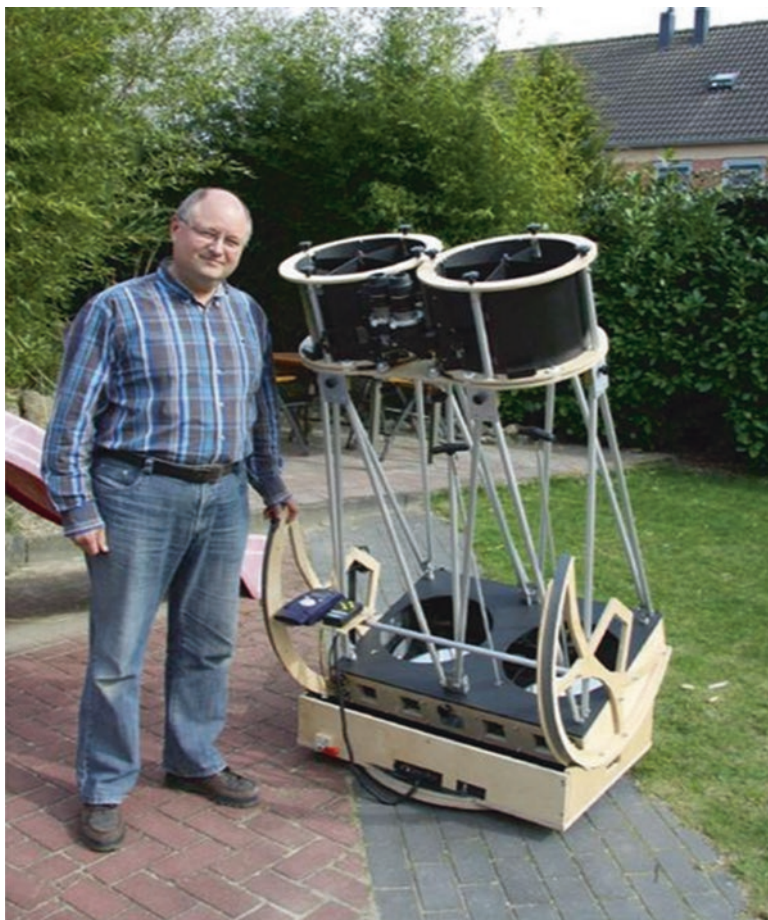
Fig. 5.46 Arie Otte of the Netherlands has made a very nice, stable looking tube truss 13-in. f/5 binocular telescope on an Altazimuth mounting (Image credit: Arie Otte)
