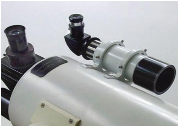
Fig. 9.1 Typical right-angle 8× power finderscope attached to a telescope (Image credit: Halfblue-Wikimedia Commons)
