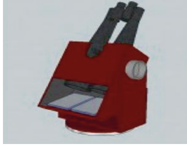
Fig. 3.12 Here is Carl’s drawing of his binocular mirror mount showing the dual mirror system (Image credit: Carl Vehmeyer)
