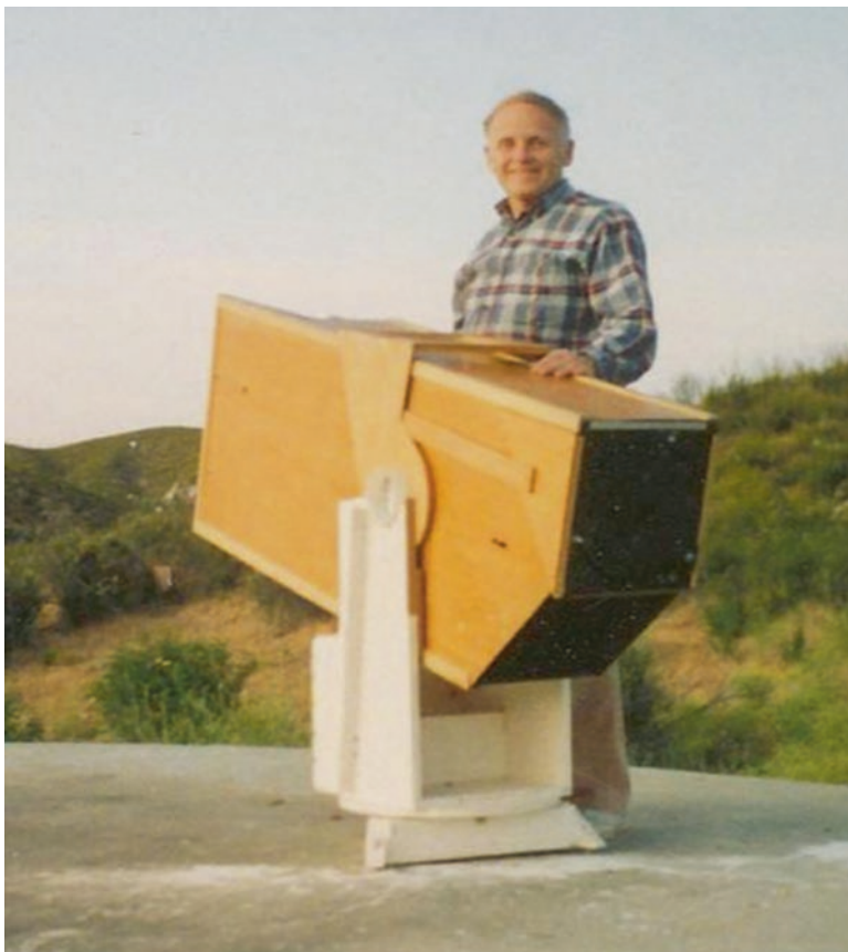
Fig. 5.43 Jim Carlisle made this very unique patented homemade all-wood 10-in. Herschel binocular telescope on an Altazimuth mounting that won a merit award at the 1992 RTMC. This is a splendidly crafted example of a homemade Herschel binocular telescope (Image credit: Jim Carlisle)
