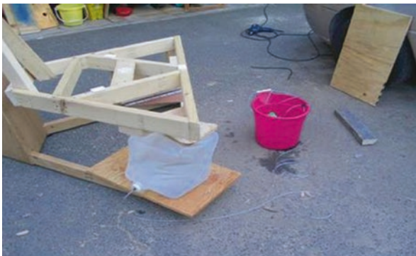
Fig. 8.33 Preliminary fluid drive uses a five gallon water bag for test purposes (Image credit: Dann McCreary)
