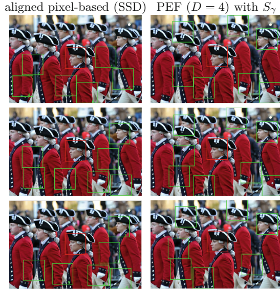
Fig. 1. Comparison of PEFPM with the baseline SSD patch matching (patch size 150 \times 150 and image size 960 \times 640 ): Observe that due to its flexibility the statistical modeling got more face hits (4 faces) than the pixel-aligned SSD method (one face). The upper row is on pixel intensities, the middle row on sum of RGB channel dissimilarities, and the last row on the maximum of RGB channel dissimilarity. (Color figure online)
