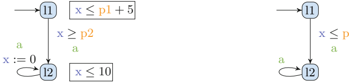
(a) PTA deadlocked for some valuations (b) PTA deadlocked for all valuations
