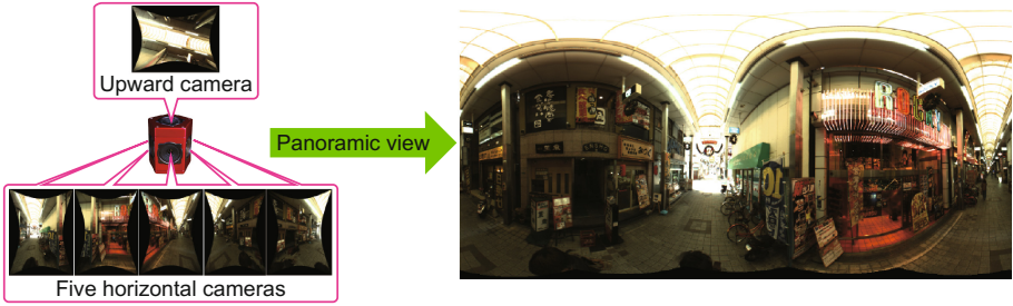
Fig. 1. Point Grey Ladybug3, an omnidirectional camera, captures six images consisting of five horizontal and one upward cameras at once. A panoramic view can be created from the six images.
