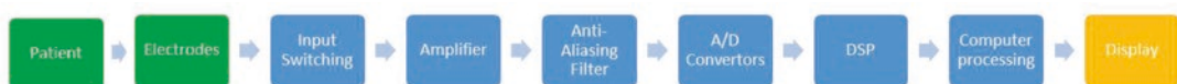
Fig. 16.9 Signal pathway of signal acquisition from the patient to the IOM equipment display
