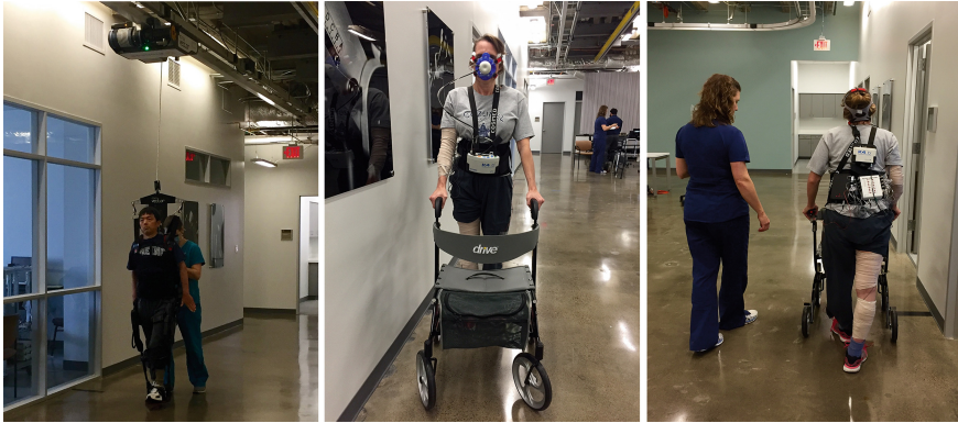
Fig. 1 Exoskeleton assisted training and assessment sessions. One subject walked with exoskeleton with body weight support system (Vector Gait and Safety System®, Bioness, left). Metabolic and EMG data collection during exoskeleton assisted walking (center and right)
