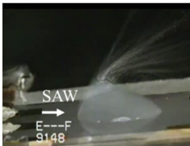
Fig. 3 Nonlinear phenomena, SAW streaming, caused by the longitudinal wave radiated from the SAW. a Droplet manipulation, b droplet ejection, and c pump
