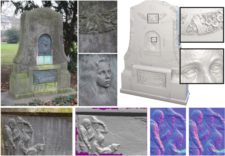
Fig. 7. Results on an outdoor dataset. Top: Input images at different scales, and our global model with details. Our method recovers more detail in regions that are imaged at higher-resolution. Bottom: A closeup input image; the reconstructed depth map shaded with the lighting; and close-up normals with regular ( 10^{-2} ) and low ( 10^{-4} ) value for \alpha – decreasing the weight of the shading term results in more noise and less detail as the stereo term dominates the energy.
