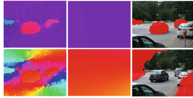
Fig. 7. RANSAC vs. no RANSAC. Top row: robust initialization with RANSAC. Bottom row: using Bruss and Horn’s method directly on the entire image. Left to right: flow angles of observed translational flow, angle field M of static environment and segmentation.
