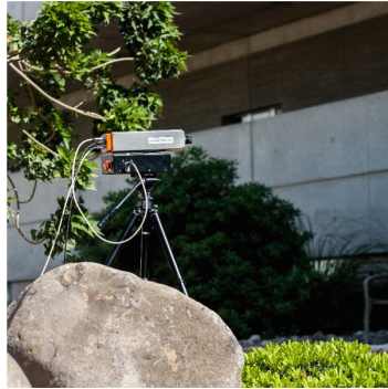
Fig. 2. The experimental setup used for the acquisition of our database includes a Specim hyperspectral camera, a computer control rotary stage mounted on a heavy duty tripod, and acquisition computer.
