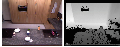
Fig. 2. The interference of multiple RGB-D cameras results in noisy depth data as seen on right. Gray areas have a valid depth, while the black regions do not provide any information about depth.
