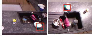
Fig. 8. A wrong detection. Bowl is detected as a cup.
