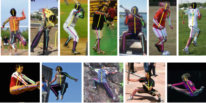
Fig. 6. Additional results of our model’s predicted joint positions on the LSP database test-set [12]
