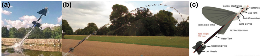
Fig. 3 a AquaMAV launching out of the water using a burst of water jet thrust. b Timelapse of a launch from water, with wings deployed in final snapshot. c CAD Renderings of the AquaMAV, all images reused from [36]
