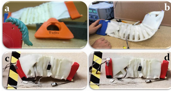
Fig. 3 The Softworm motor-tendon technology has been applied to power a large (60 cm) robot constructed from plastic foam. A living caterpillar is shown in a together with motor housings and the body. b shows the robot lifting its “head” and c and d show stages of a single “step” during the RoboSoft Grand Challenge Competition. Photos courtesy of the Tufts RoboSoft Team
