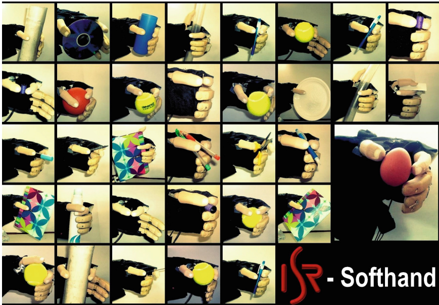
Fig. 1 ISR-Softhand can perform 31 grasps out of the 33 grasps that humans achieve on their daily activities
