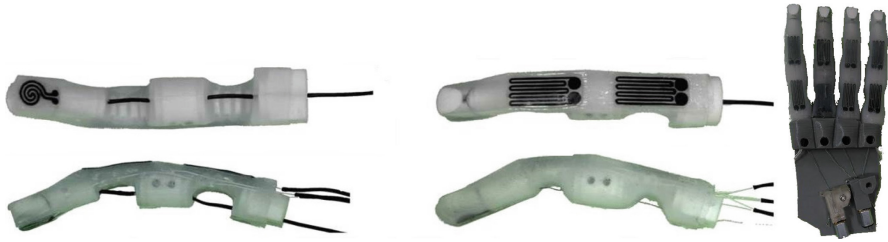
Fig. 5 An electronic skin composed of soft pressure sensors and bend sensors are embedded on the digits of soft-hand
