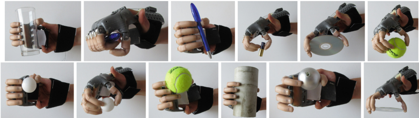
Fig. 4 Body-actuated hand with soft digits
