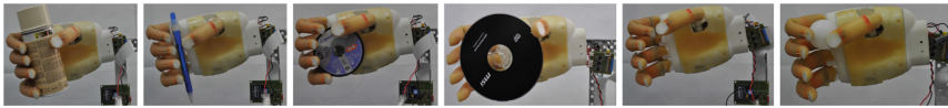
Fig. 3 UC-Soft hand has an independent actuator dedicated for rotation of the thumb
