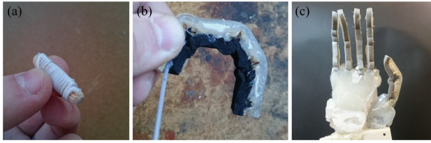
Fig. 4 In this design, links are made of wood which carry the pulleys that allow the translation of actuator force through the fingers (a). Wood links are connected to each other with soft HMA material to form soft joints and contribute to the overall flexibility of the manipulator. Finger pads are covered with soft sponge materials to assist form closure (b). By repeating the same finger design, a hybrid manipulator that resembles the human hand is created. Palm is reinforced with rigid materials for the fingers to apply necessary forces during grasping (c)
